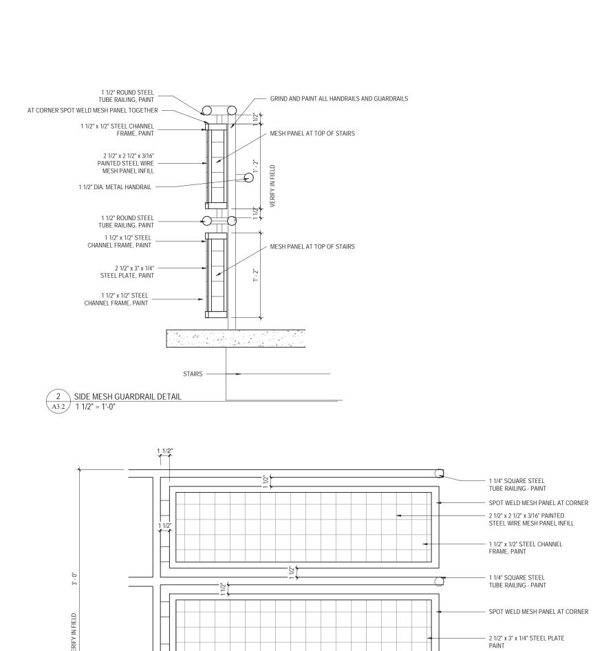
3 MESH GUARDRAIL DETAIL
