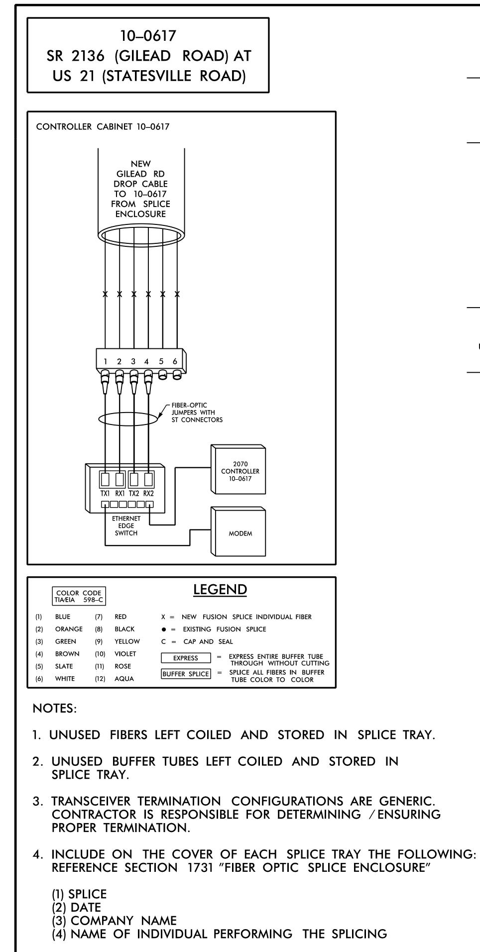
PRIOR TO INSTALLING THE COVER ON THE SPLICE TRAY, TAKE A DIGITAL PHOTOGRAPH SHOWING THE SPLICE TRAY AND INFORMATION SHOWN ABOVE (1-4) AND SUBMIT PHOTOGRAPH ALONG WITH OTDR TEST RESULTS.
