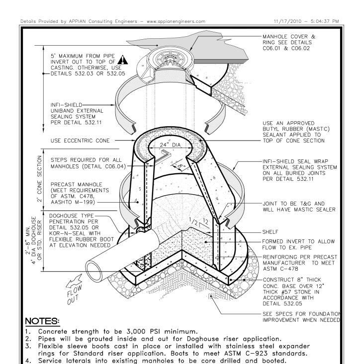
For watertight applications, place butyl rubber between frame and cone with
