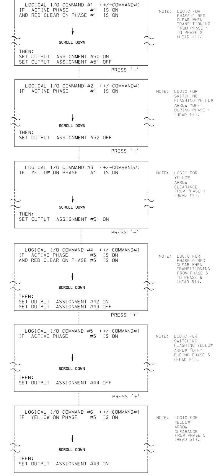
**OUTPUT REFERENCE SCHEDULE** USE TO INTERPRET LOGIC PROCESSOR OUTPUT 42 = Overlap C Red OUTPUT 43 = Overlap C Yellow OUTPUT 44 = Overlap C Green OUTPUT 50 = Overlap A Red OUTPUT 51 = Overlap A Yellow OUTPUT 52 = Overlap A Green
