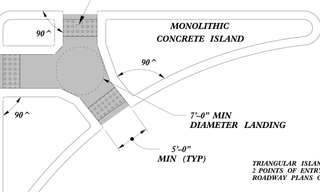
TRIANGULAR ISLANDS MAY BE CONSTRUCTED WITH ONLY 2 POINTS OF ENTRY AND EXIT AS SHOWN IN THE ROADWAY PLANS OR AS DIRECTED BY THE ENGINEER.
