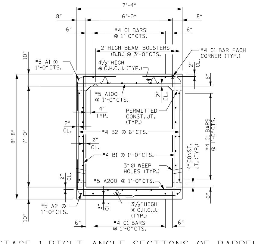
\* ALL CONTINUOUS HIGH CHAIR UPPER (C.H.C.U.) @ 3'-0"CTS. THERE ARE 32 C1 BARS (3 BAR RUN) IN SECTION OF BARREL
