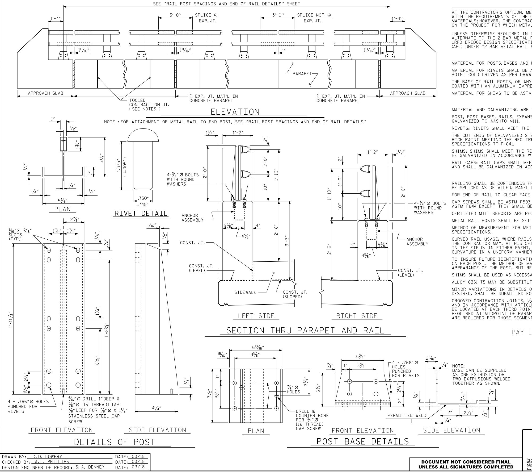
AT THE CONTRACTOR'S OPTION, METAL RAIL MAY BE EITHER ALUMINUM OR GALVANIZED STEEL IN ACCORDANCE WITH THE REQUIREMENTS OF THE GENERAL NOTES AND THE FOLLOWING SPECIFICATIONS FOR THE ALTERNATE MATERIALS; HOWEVER, THE CONTRACTOR WILL BE REQUIRED TO USE THE SAME RAIL MATERIAL ON ALL STRUCTURES ON THE PROJECT FOR WHICH METAL RAIL IS DESIGNATED.
