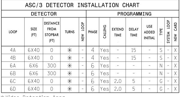
\*Video Detection Area Camra locations should be confirmed in the field by the contractor in order to provide detection of the areas indicated.
