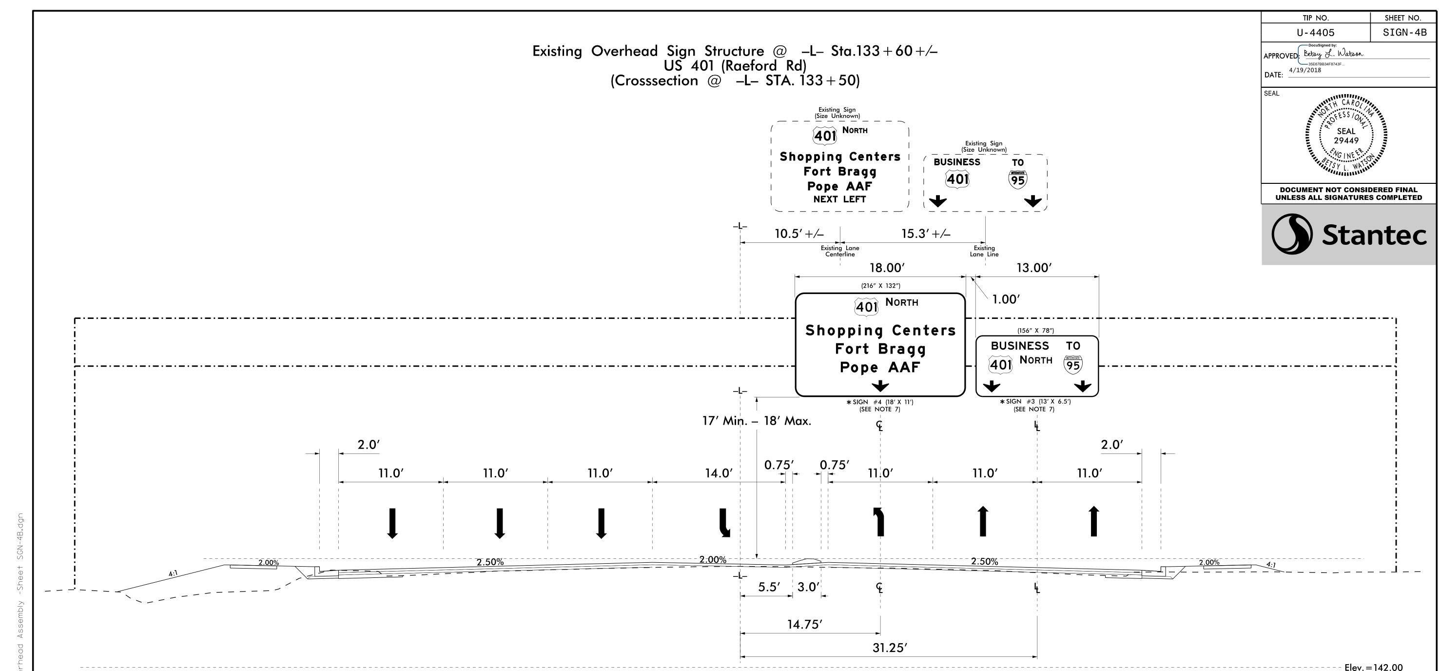
The contractor shall verify that the total square footage of new signs #3 and #4 does not exceed the square footage of the existing signs being removed from this overhead structure.
