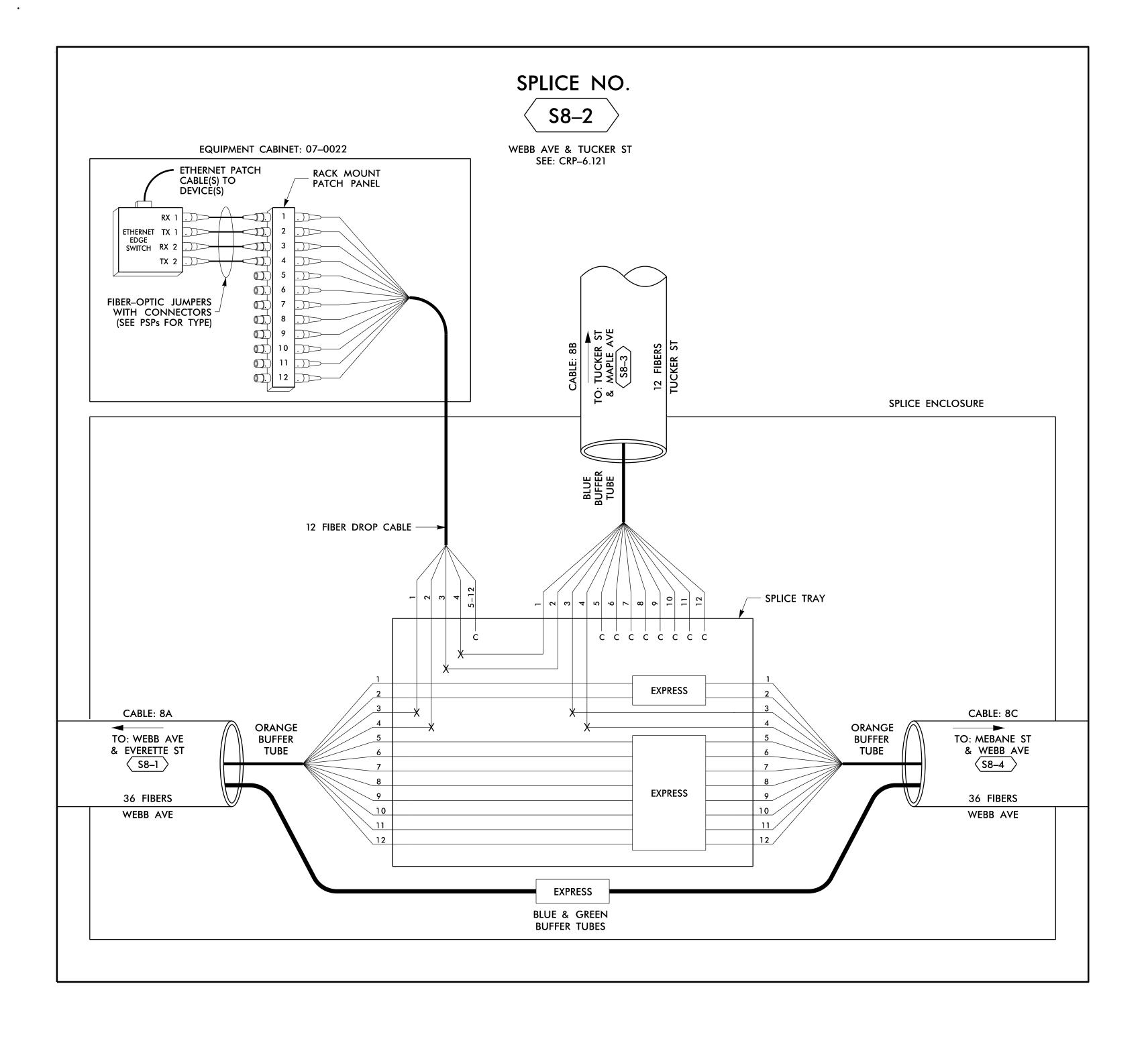
**LEGEND NOTES** X = FUSION SPLICE INDIVIDUAL FIBER1. UNUSED FIBERS LEFT COILED AND STORED IN SPLICE TRAY C = CAP AND SEAL2. UNUSED BUFFER TUBES LEFT COILED AND STORED IN SPLICE ENCLOSURE EXPRESS ENTIRE BUFFER TUBE /FIBERS **EXPRESS** 3. EDGE SWITCH CONFIGURATIONS ARE GENERIC. CONTRACTOR IS RESPONSIBLE FOR DETERMINING/ENSURING THE PROPER TERMINATIONS. THROUGH WITHOUT CUTTING SPLICE ALL FIBERS IN BUFFER TUBE COLOR TO COLOR
