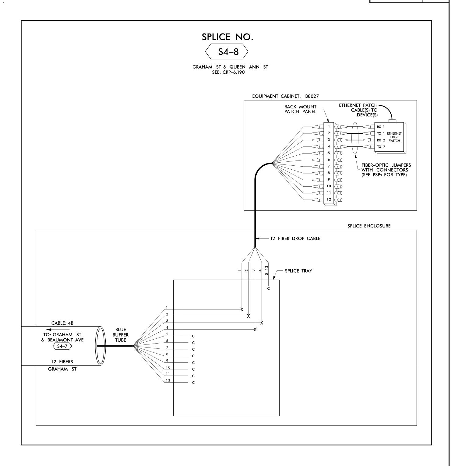
**LEGEND NOTES** X = FUSION SPLICE INDIVIDUAL FIBER1. UNUSED FIBERS LEFT COILED AND STORED IN SPLICE TRAY C = CAP AND SEAL2. UNUSED BUFFER TUBES LEFT COILED AND STORED IN SPLICE ENCLOSURE EXPRESS ENTIRE BUFFER TUBE /FIBERS **EXPRESS**
