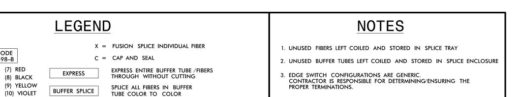
EXISTING BUFFER TUBE /FIBERS. DO NOT
