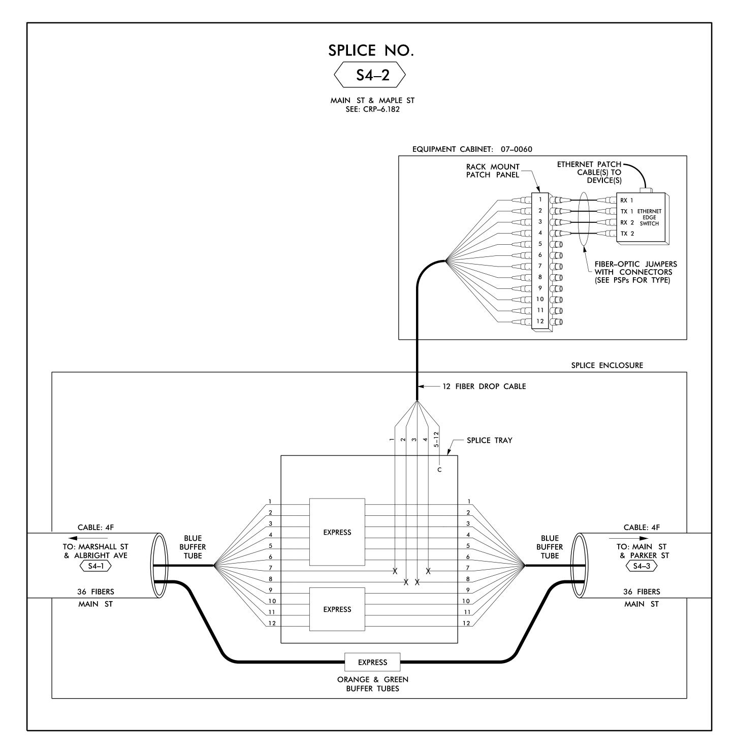
**LEGEND NOTES** X = FUSION SPLICE INDIVIDUAL FIBER1. UNUSED FIBERS LEFT COILED AND STORED IN SPLICE TRAY C = CAP AND SEAL2. UNUSED BUFFER TUBES LEFT COILED AND STORED IN SPLICE ENCLOSURE **EXPRESS**
