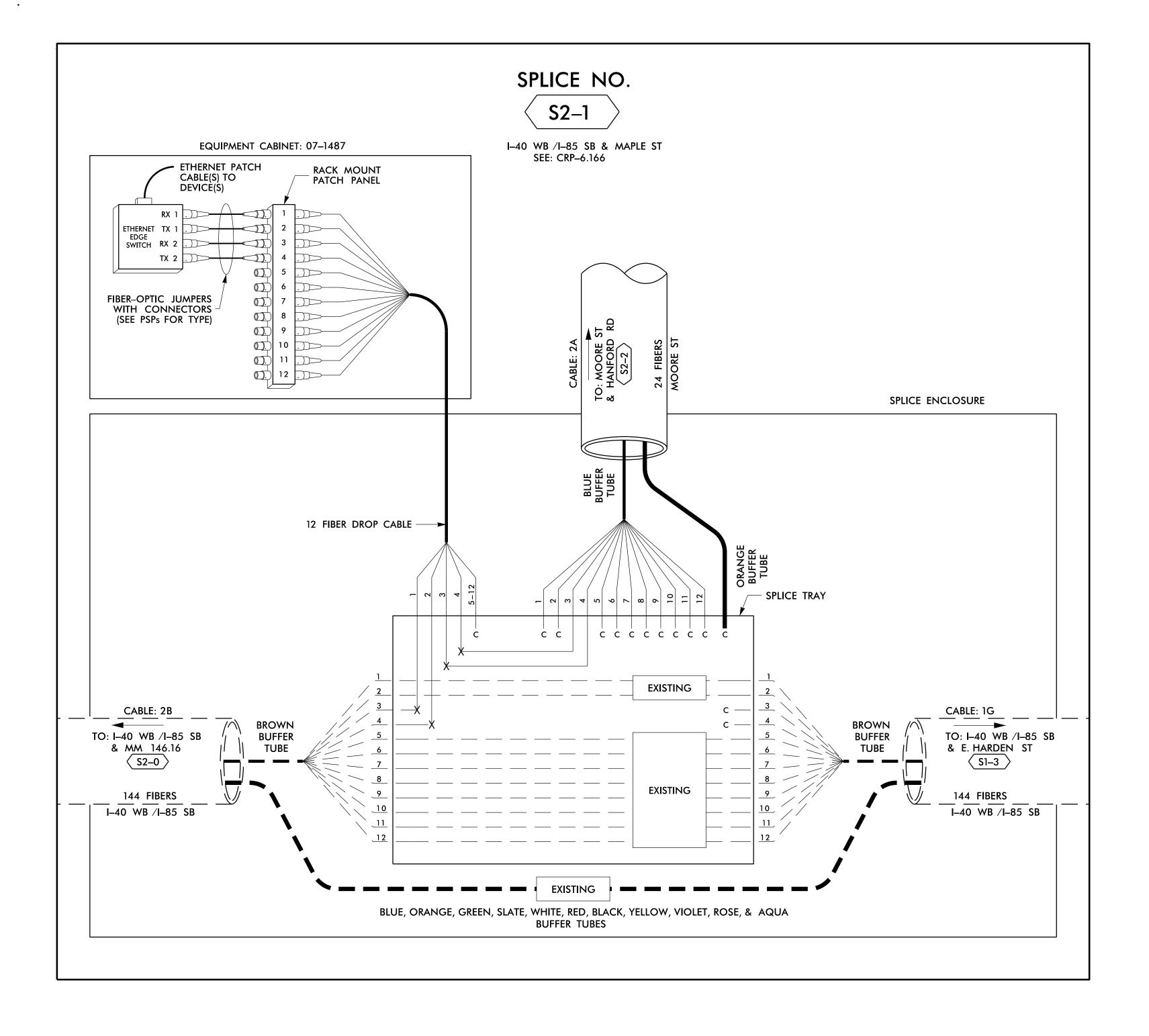
**LEGEND NOTES** X = FUSION SPLICE INDIVIDUAL FIBER1. UNUSED FIBERS LEFT COILED AND STORED IN SPLICE TRAY C = CAP AND SEAL2. UNUSED BUFFER TUBES LEFT COILED AND STORED IN SPLICE ENCLOSURE EXPRESS ENTIRE BUFFER TUBE /FIBERS **EXPRESS** 3. EDGE SWITCH CONFIGURATIONS ARE GENERIC. CONTRACTOR IS RESPONSIBLE FOR DETERMINING/ENSURING THE PROPER TERMINATIONS. THROUGH WITHOUT CUTTING
