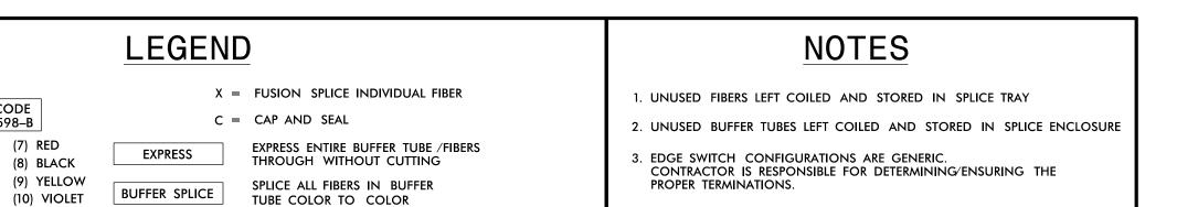
EXISTING BUFFER TUBE /FIBERS. DO NOT
