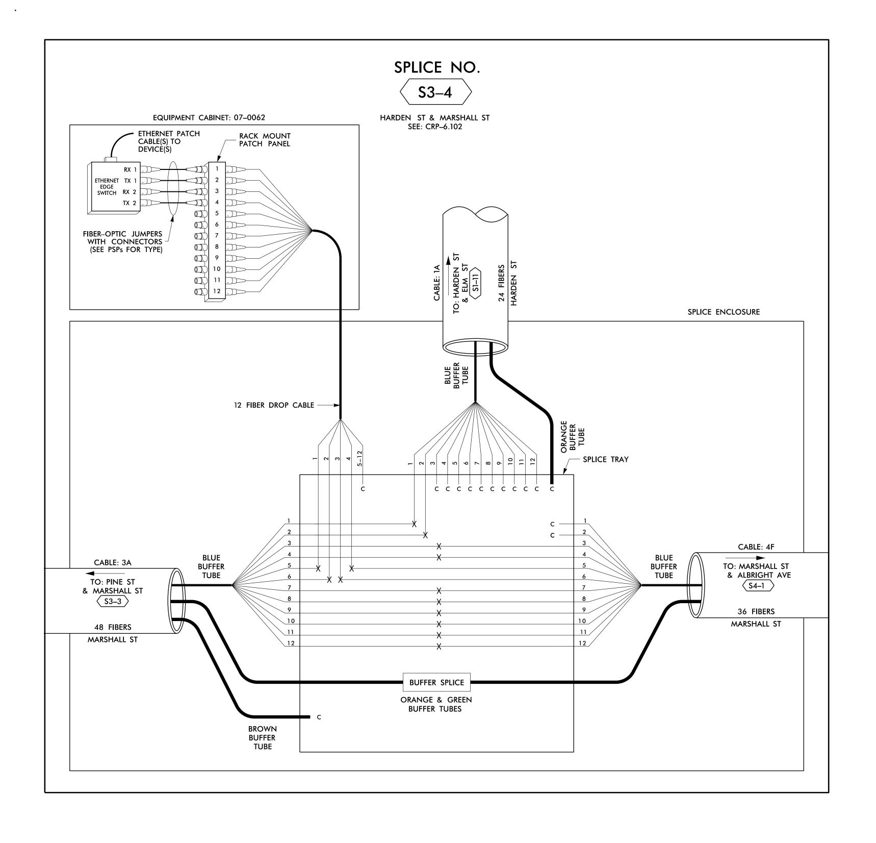
**LEGEND** X = FUSION SPLICE INDIVIDUAL FIBERC = CAP AND SEALEXPRESS ENTIRE BUFFER TUBE /FIBERS **EXPRESS** THROUGH WITHOUT CUTTING
