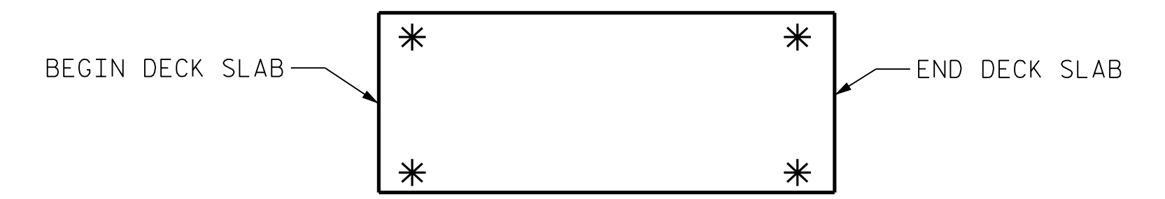
SKETCH SHOWING POINTS OF ATTACHMENTS * DENOTES GUARDRAIL ANCHOR ASSEMBLY
