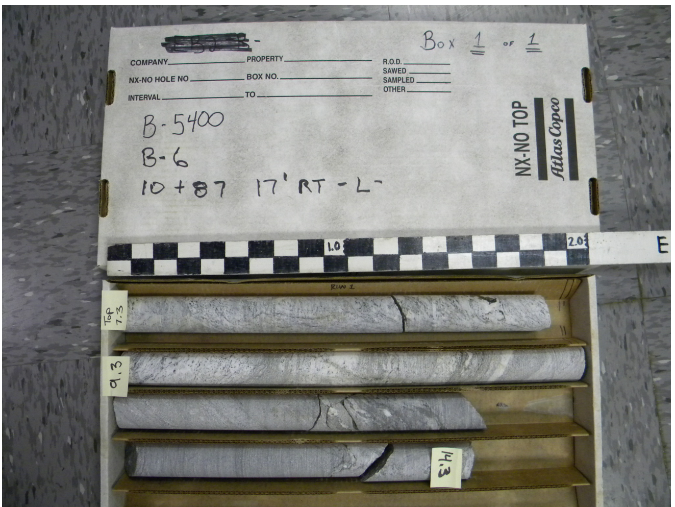
B-5400 BORING B-6 STATION 10+87 17' RT 7.5 TO 14.3 BLOCK GOOD TO VERY GOOD GNEISS GSI = 75 - 85
