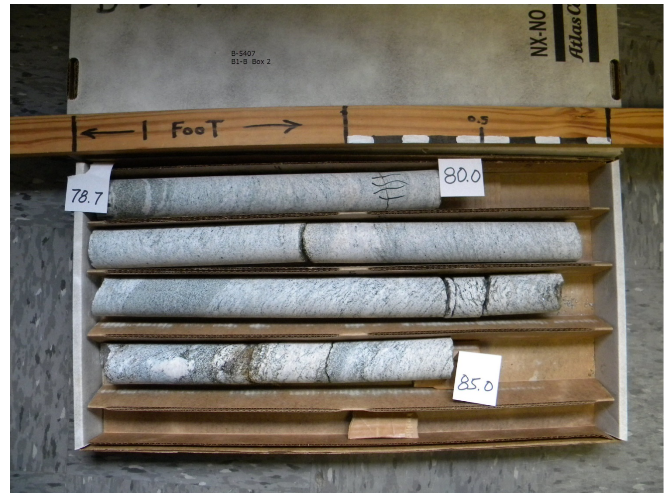
B-5407 BORING B1-B BOX 2 OF 2 DEPTH: 78.7-85.0
