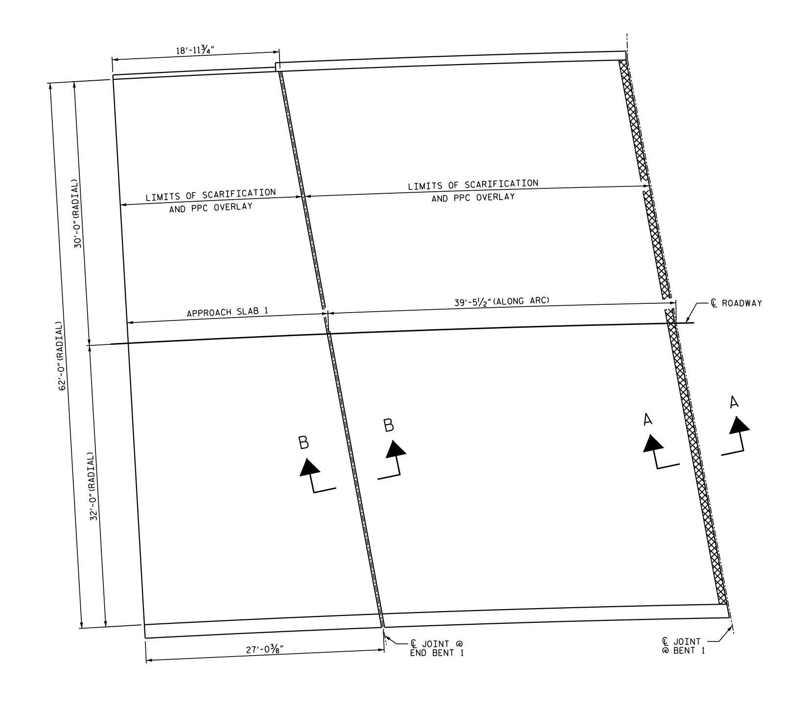
AS-BUILT REPAIR QUANTITY TABLE TOP OF DECK REPAIRS ESTIMATE ACTUAL SCARIFYING BRIDGE DECK 430 SQ. YDS. CLASS II SURFACE PREPARATION 7.0 SQ. YDS. 7.0 SQ. YDS. CONCRETE DECK REPAIR FOR PPC OVERLAY SHOTBLASTING BRIDGE DECK 430 SQ. YDS. 14.9 CU. YDS. PPC MATERIALS 430 SQ. YDS. PLACING AND FINISHING PPC OVERLAY
