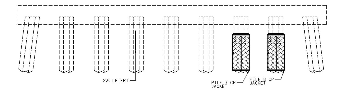
QUANTITIES BENT 33 ACTUAL ESTIMATE VOLUME CU.FT. VOLUME CU.FT. AREA SQ.FT. AREA SQ.FT SHOTCRETE REPAIRS CAP 3.2 COLUMN/PILE 1.6 AREA SQ.FT CONCRETE REPAIRS CAP EPOXY RESIN INJECTION LIN.FT. LIN.FT CAP COLUMN/PILE 5.0 PILE REPAIR JACKET LIN.FT. LIN.FT 14.0 GALVANIC STRUCTURAL C.P. JACKET
