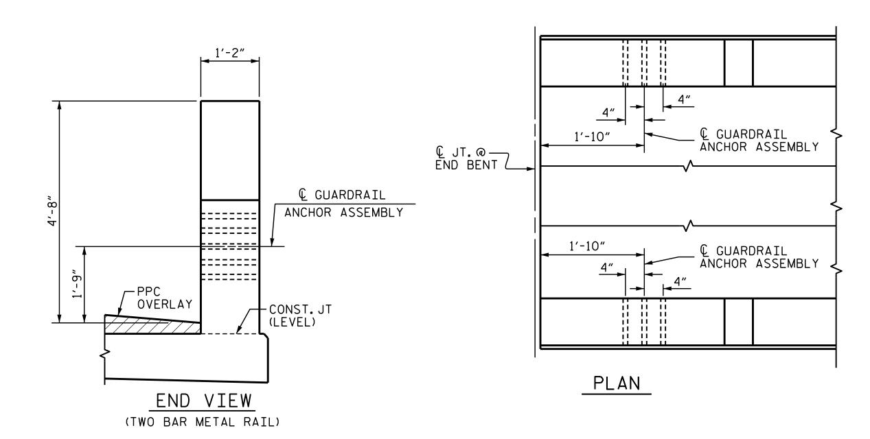
LOCATION OF GUARDRAIL ANCHOR AT END POST
