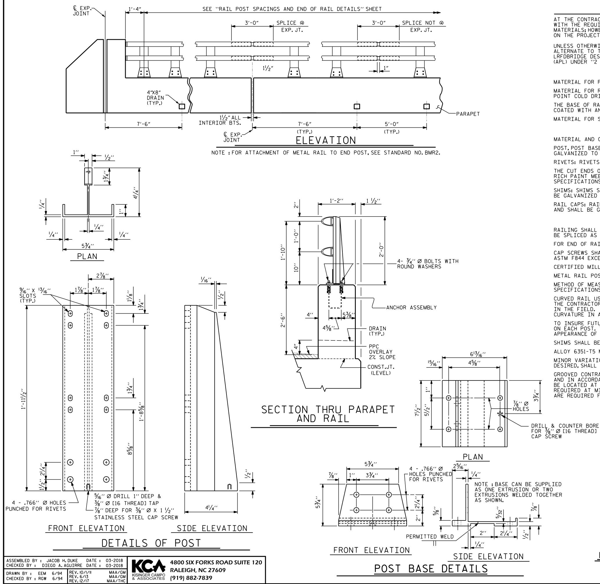
AT THE CONTRACTOR'S OPTION, METAL RAIL MAY BE EITHER ALUMINUM OR GALVANIZED STEEL IN ACCORDANCE WITH THE REQUIREMENTS OF THE GENERAL NOTES AND THE FOLLOWING SPECIFICATIONS FOR THE ALTERNATE MATERIALS; HOWEVER, THE CONTRACTOR WILL BE REQUIRED TO USE THE SAME RAIL MATERIAL ON ALL STRUCTURES ON THE PROJECT FOR WHICH METAL RAIL IS DESIGNATED.
