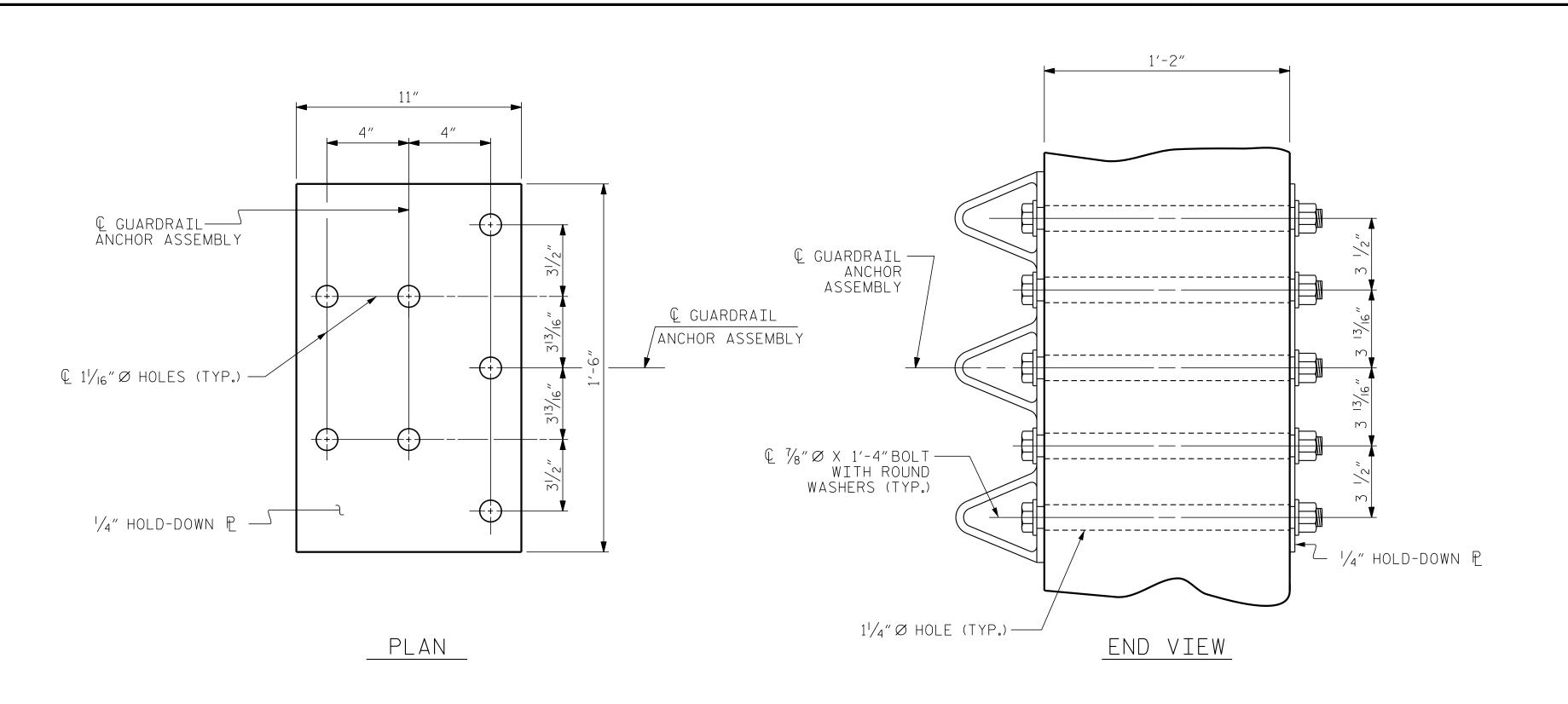
GUARDRAIL ANCHOR ASSEMBLY DETAILS
