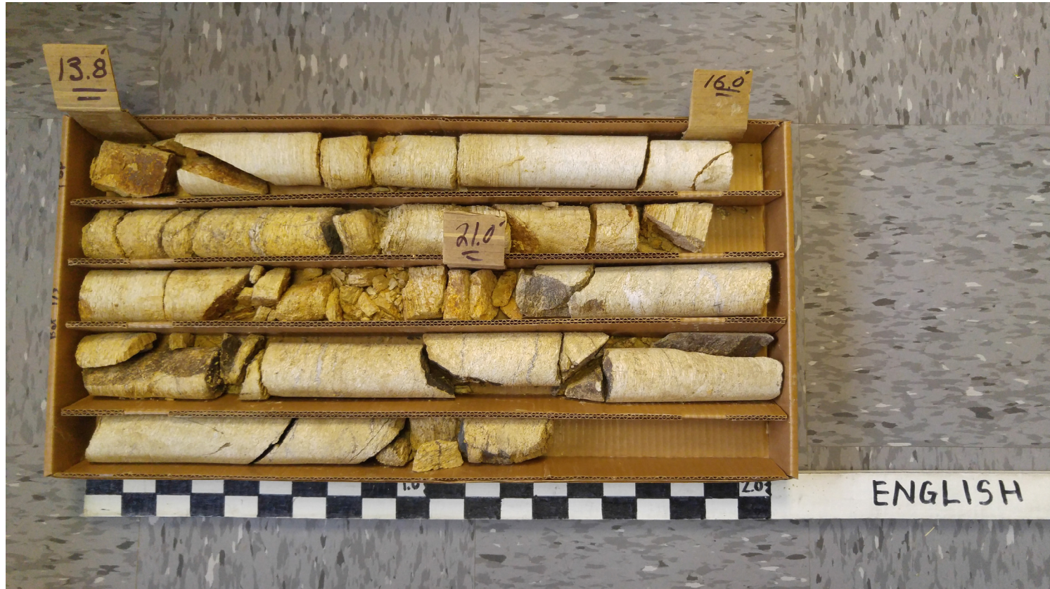
46120 (B-5405) Transylvania County Bridge No. 139 on SR-1139 Over East Branch Toxaway Creek Boring EB-1B Box 1 of 3 Depth: 13.8' – 25.0'
