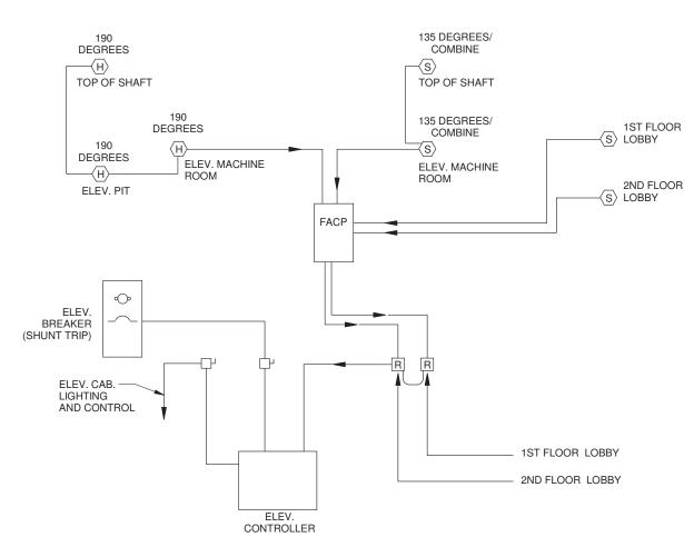
3 ELEVATOR RECALL AND DETECTION DETAIL 1)
