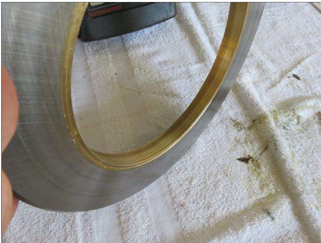
NORTH EAST ROOM INNER SOUTH SIDE BRONZE BUSHING HAS 1/32" GROOVES IN BRONZE RING.
