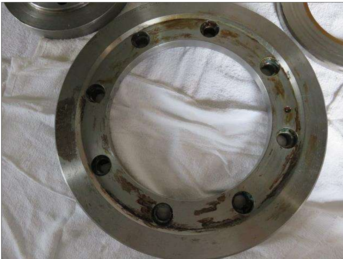
SOUTH WEST ROOM SOUTH SIDE TRUNNION INNER PLATE HAS AREAS OF SURFACE RUST ON FACE. (NO SECTION LOSS PRESENT)
