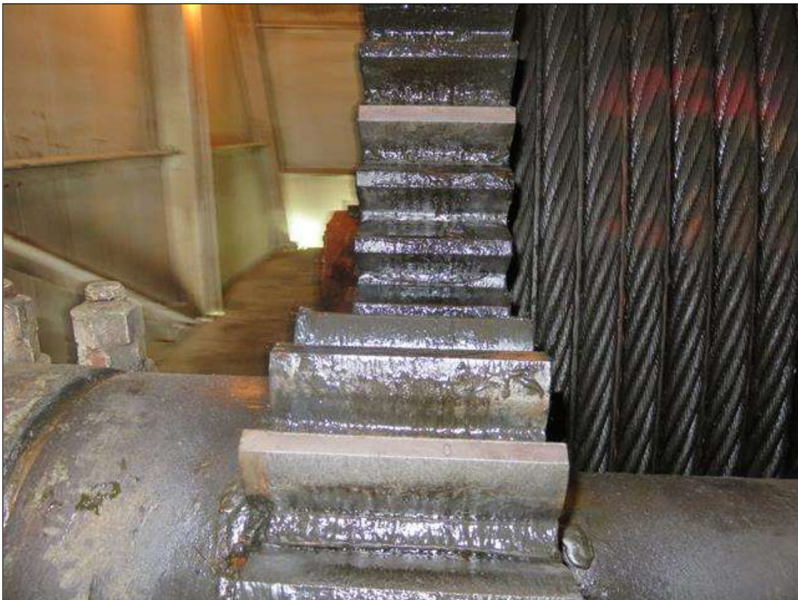
GEARS 271-1 & 276 NORTH WEST ROOM BOTH HAVE SCORING AND 1/32" GROOVES ON OPEN AND CLOSING SIDE OF TEETH.
