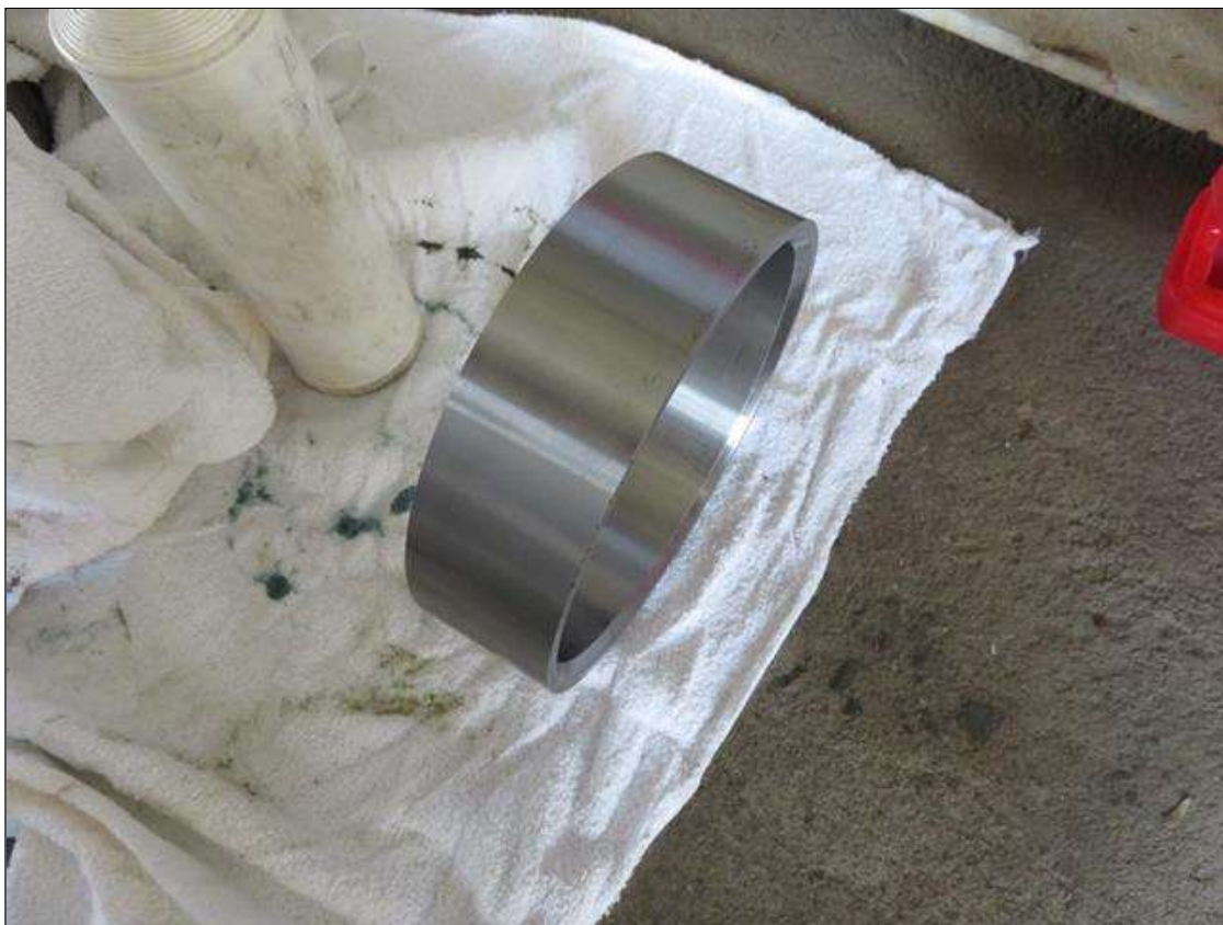
NORTH EAST ROOM INNER SOUTH SIDE TRUNNION REPLACEMENT RACE BUSHING (NEW)
