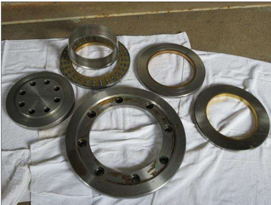
SOUTH WEST ROOM INNER TRUNNION PARTS. (GOOD)
