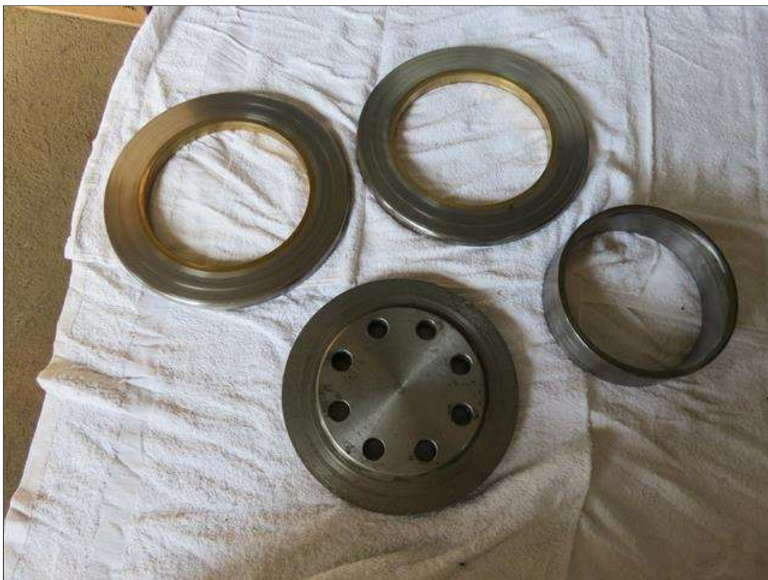
SOUTH EAST ROOM, INNER SOUTH SIDE CAP, RACE BUSHING, BRONZE BUSHINGS (NO PROBLEMS FOUND)
