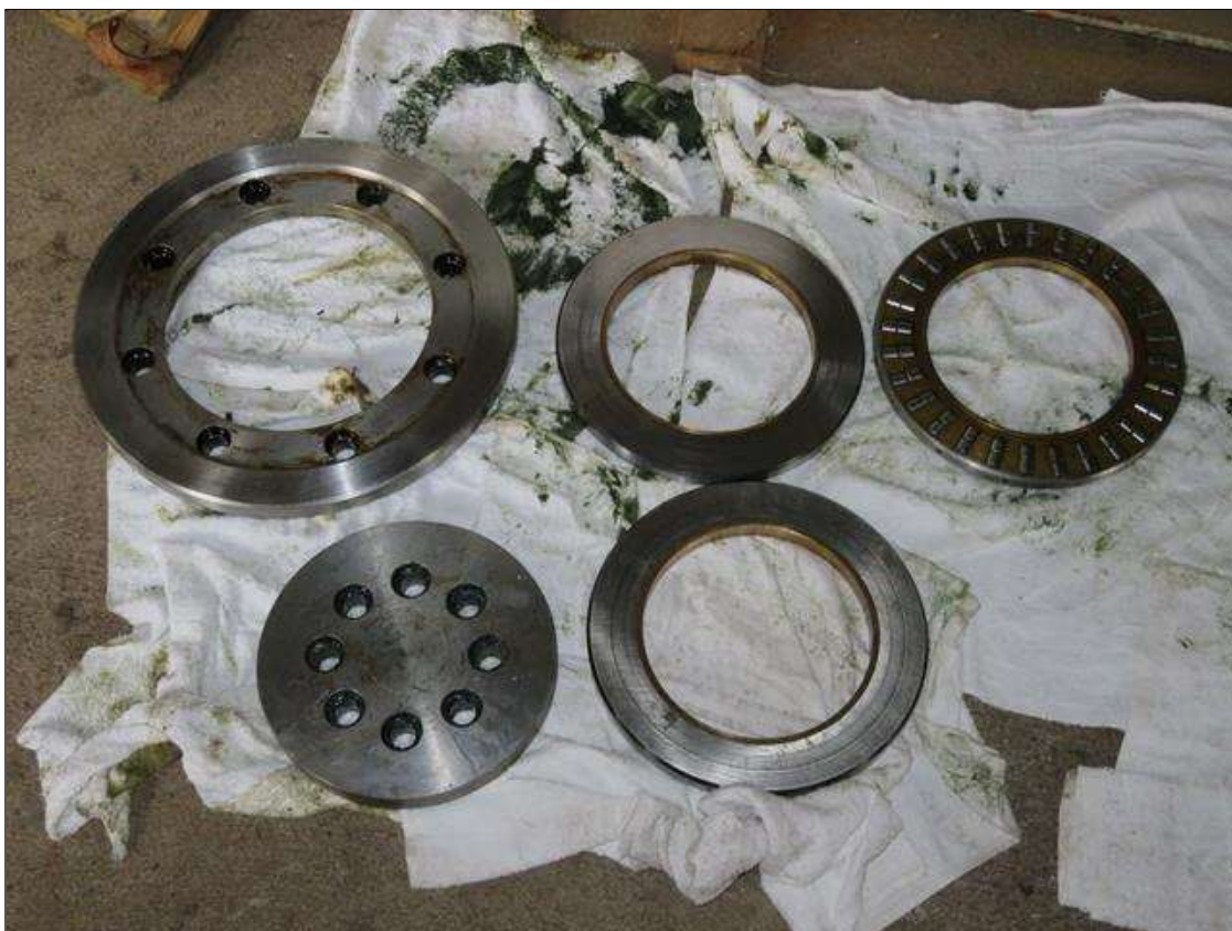
NORTH WEST ROOM INNER SOUTH TRUNNION PARTS AFTER BEING TESTED WITH ULTRA SONICS MACHINE.
