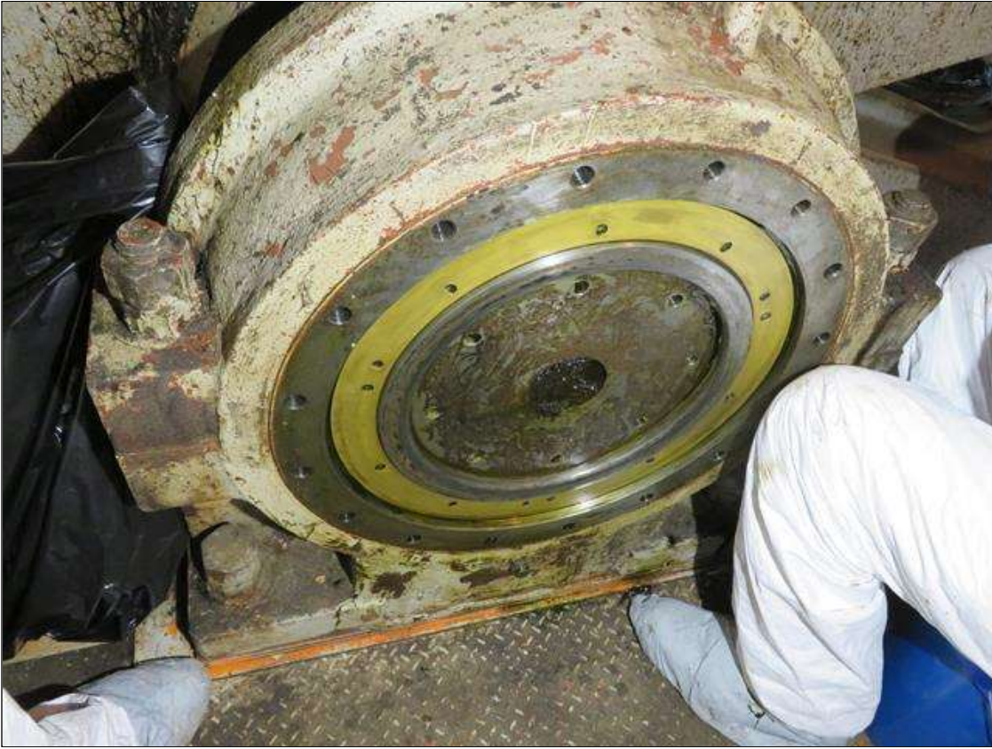
NORTH WEST ROOM OUTSIDE SOUTH TRUNNION DISASSEMBLED FOR ULTRA SONICS INSPECTION.
