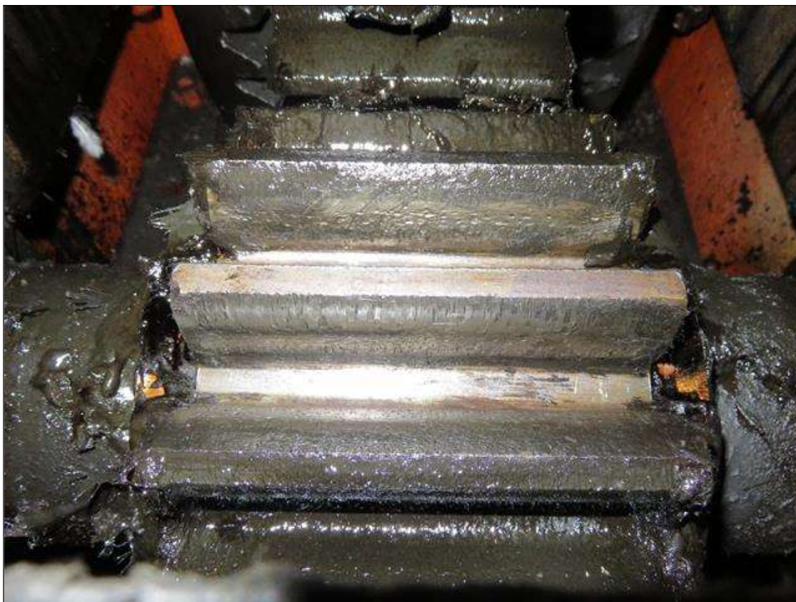
GEARS 278 HAS 1/16" DEEP GOUGES IN OPEN AND CLOSING SIDES OF TEETH.
