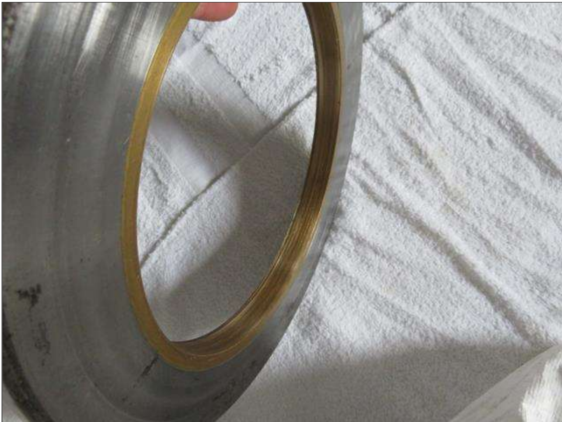
BRONZE BUSHING FROM SOUTH WEST ROOM INNER SOUTH TRUNNION HAS 1/8" DEEP GROOVES IN BRONZE RING AND WAS REPLACED WITH NEW DURING OUR 2017 INSPECTION.
