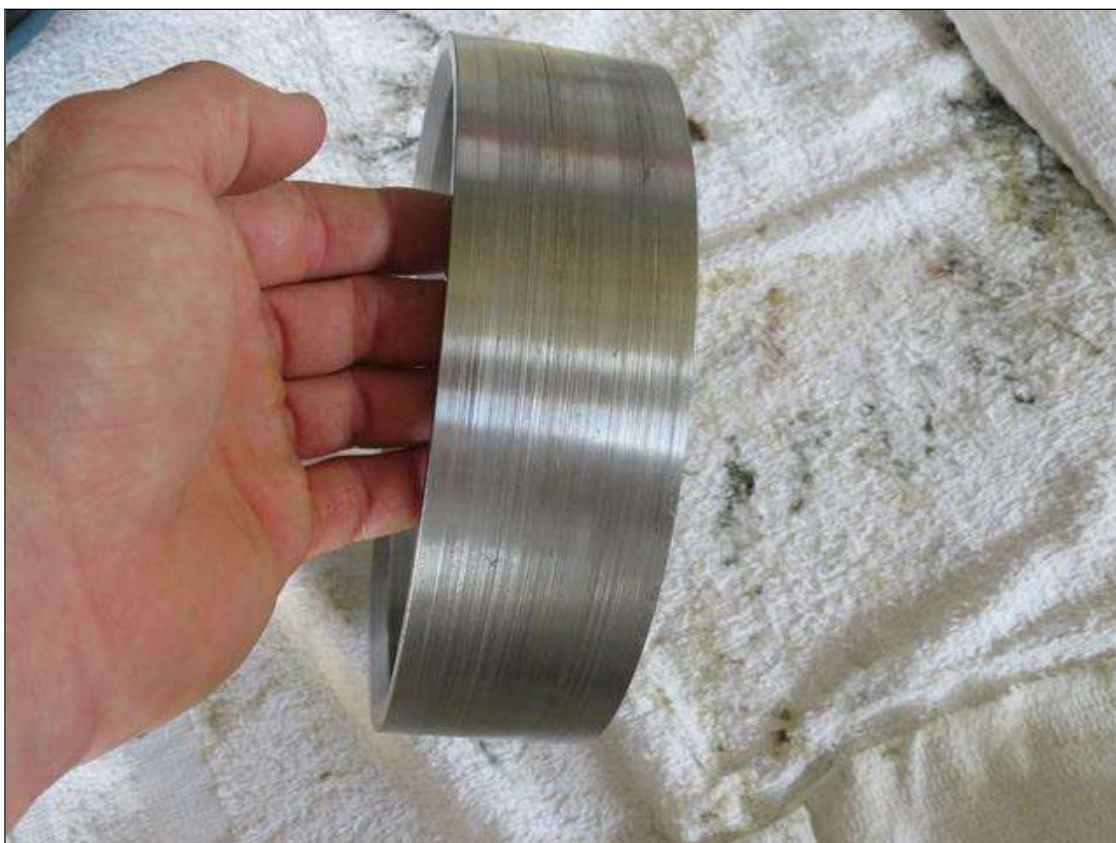
NORTH EAST ROOM INNER SOUTH SIDE RACE BUSHING HAS SEVERAL DEEP GROOVES AND IS BEING REPLACED WITH NEW DURING THE 2017 INSPECTION.
