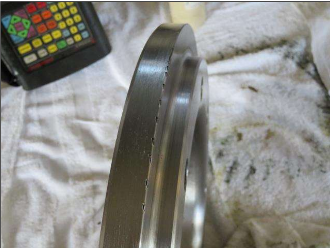
NORTH EAST ROOM SOUTH SIDE INNER PLATE HAS A SERIES OF 1/16" KNICKS ALONG EDGE FOR A LENGTH OF 9"
