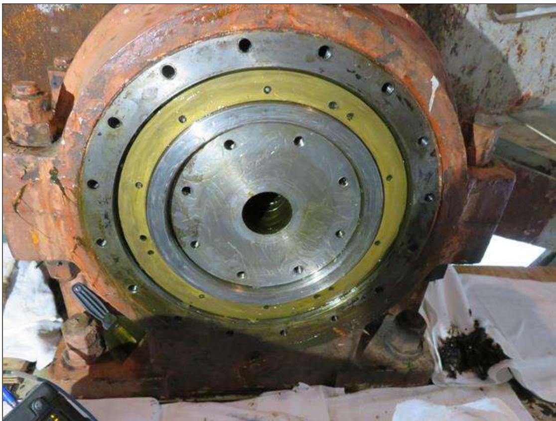
SOUTH WEST OUTSIDE TRUNNION AFTER TESTING WITH ULTRA SONICS MACHINE. (SOUTH SIDE)
