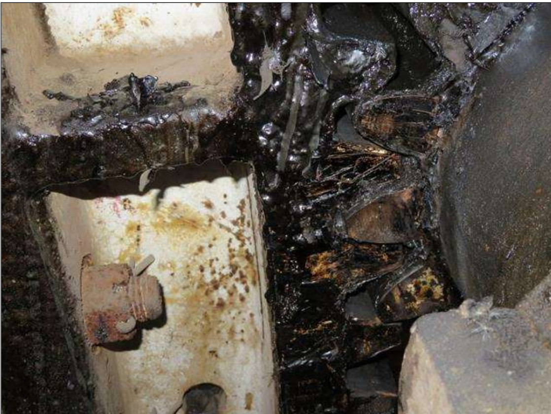
ROOT TO TIP WAS MEASURED .189 FOR GEARS 271-2 & 276 IN SOUTH WEST ROOM (WEST TOWER)
