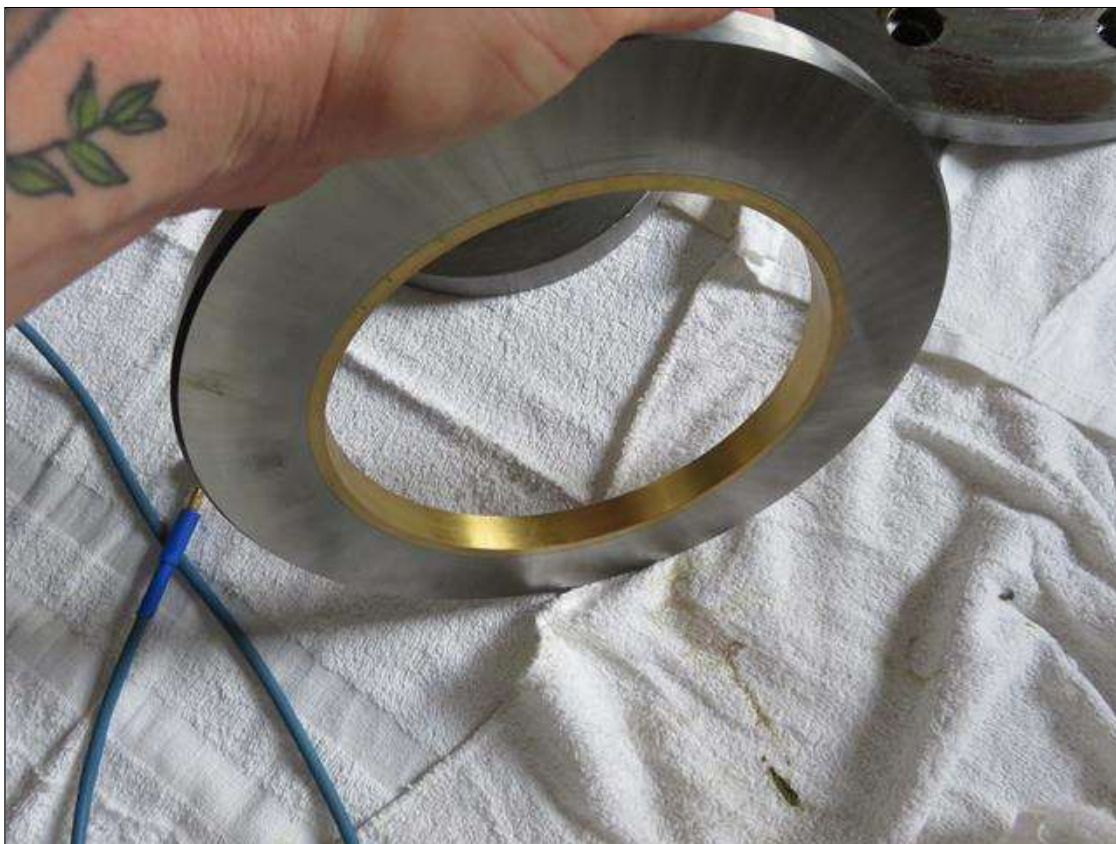
NEW BRONZE REPLACEMENT BUSHING FOR SOUTH WEST ROOM INNER SOUTH TRUNNION.
