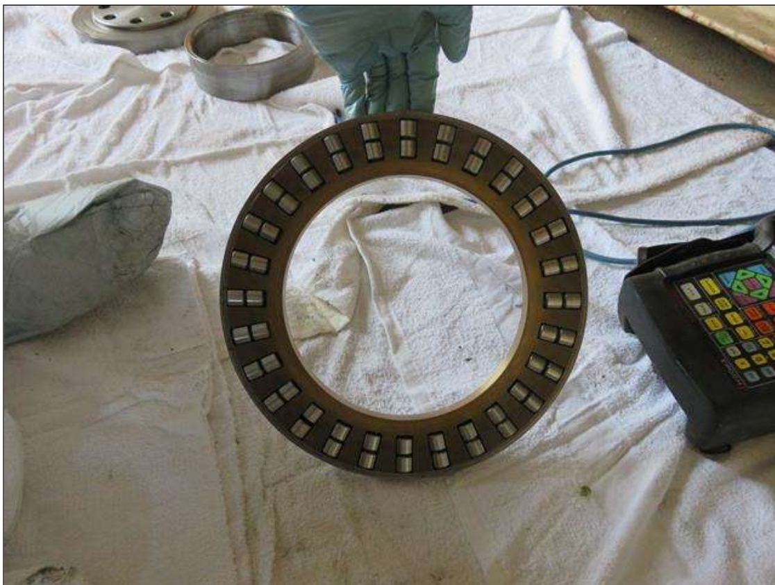
SOUTH EAST ROOM INNER SOUTH SIDE BEARING RACE (GOOD)
