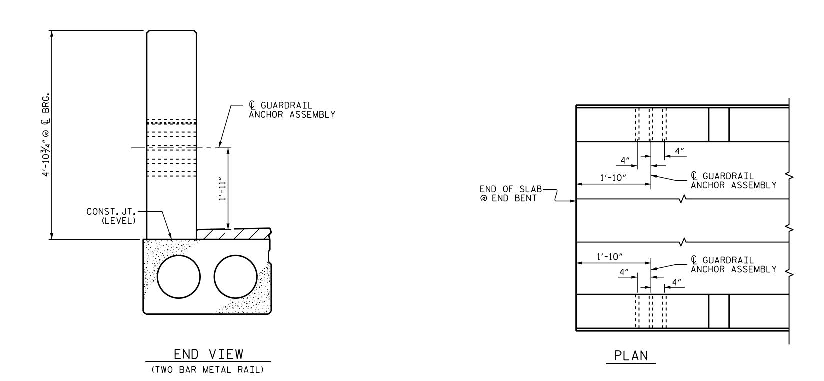
LOCATION OF GUARDRAIL ANCHOR AT END POST
