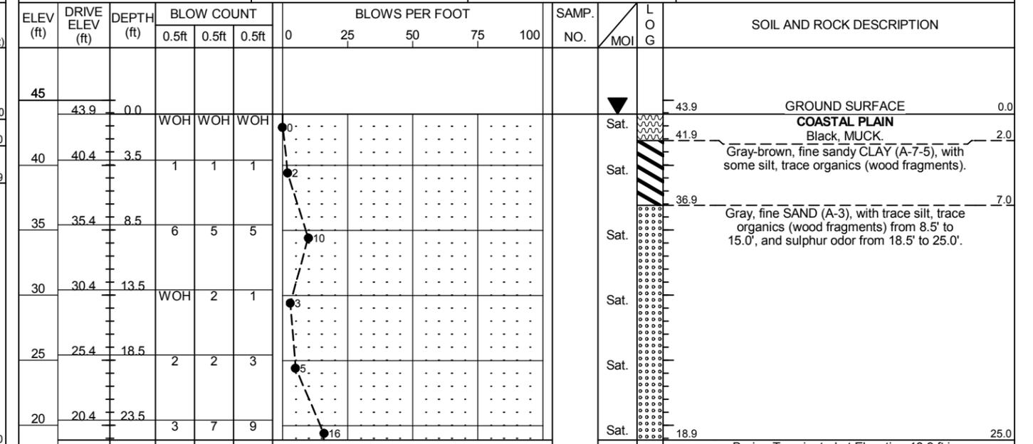
Boring Terminated at Elevation 18.9 ft in SAND (COASTAL PLAIN)
