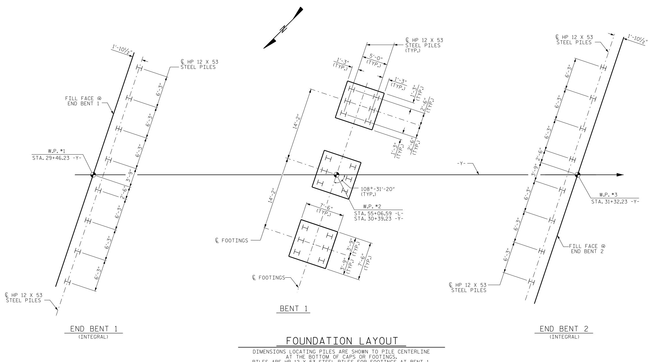
PILES ARE HP 12 X 53 STEEL PILES FOR FOOTINGS AT BENT 1. ALL PILES ARE VERTICAL.
