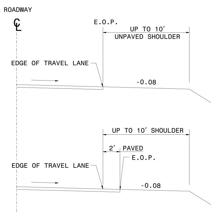
NOTE: ON LOW SIDE OF SUPERELEVATED PAVEMENT USE NORMAL SHOULDER SLOPE UNLESS NORMAL SHOULDER SLOPE IS ELEVATION RATE ON SHOULDER.
