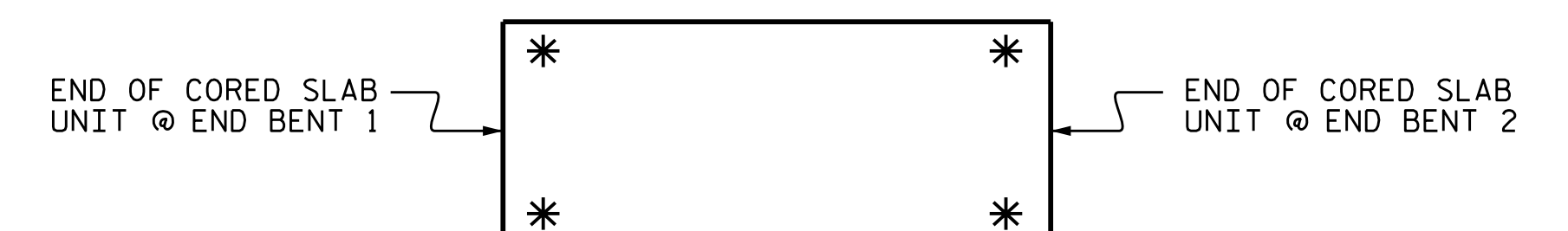
SKETCH SHOWING POINTS OF ATTACHMENT * DENOTES GUARDRAIL ANCHOR ASSEMBLY
