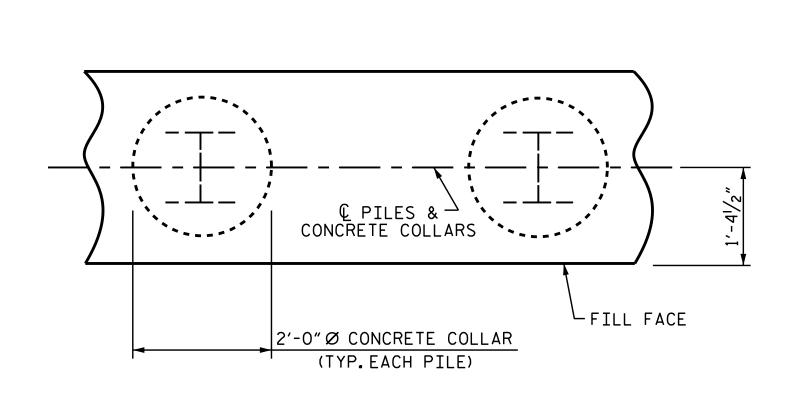
CONCRETE — COLLAR © HP 12 X 53 <u>' '</u> STEEL PILE <sub>|</sub> ELEVATION
