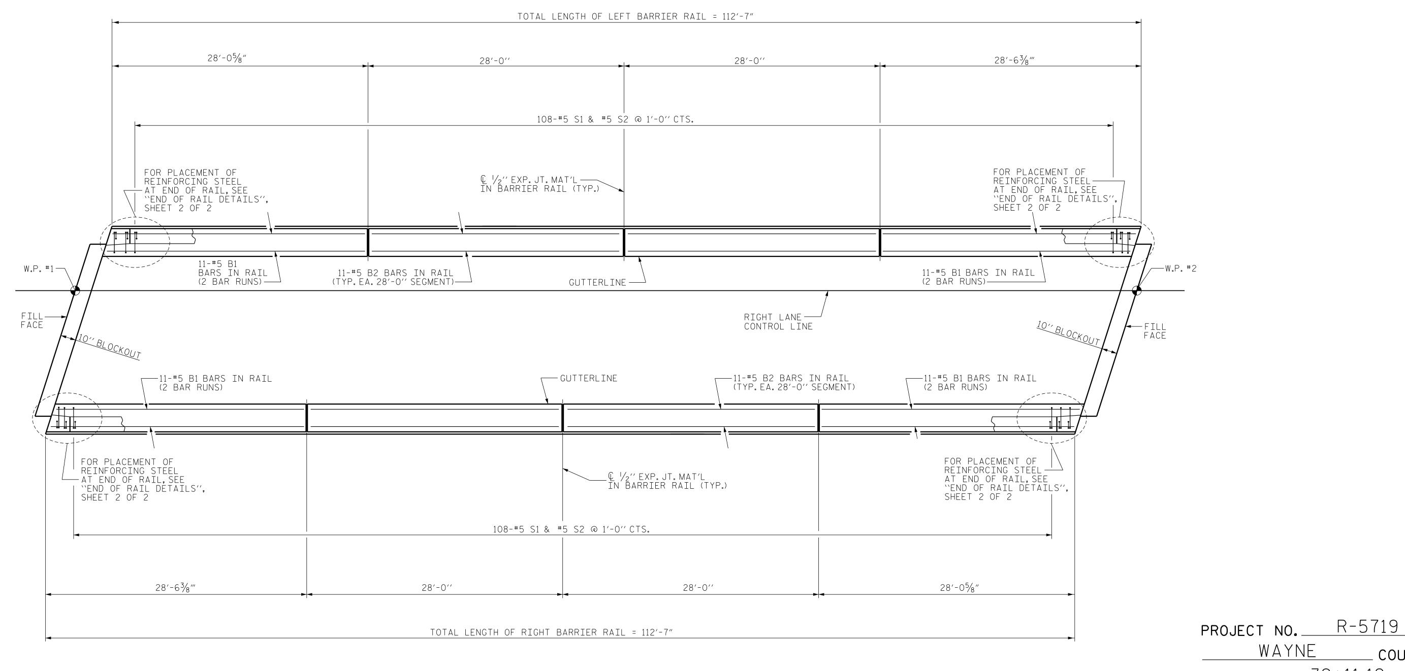
PLAN OF CONCRETE BARRIER RAIL
