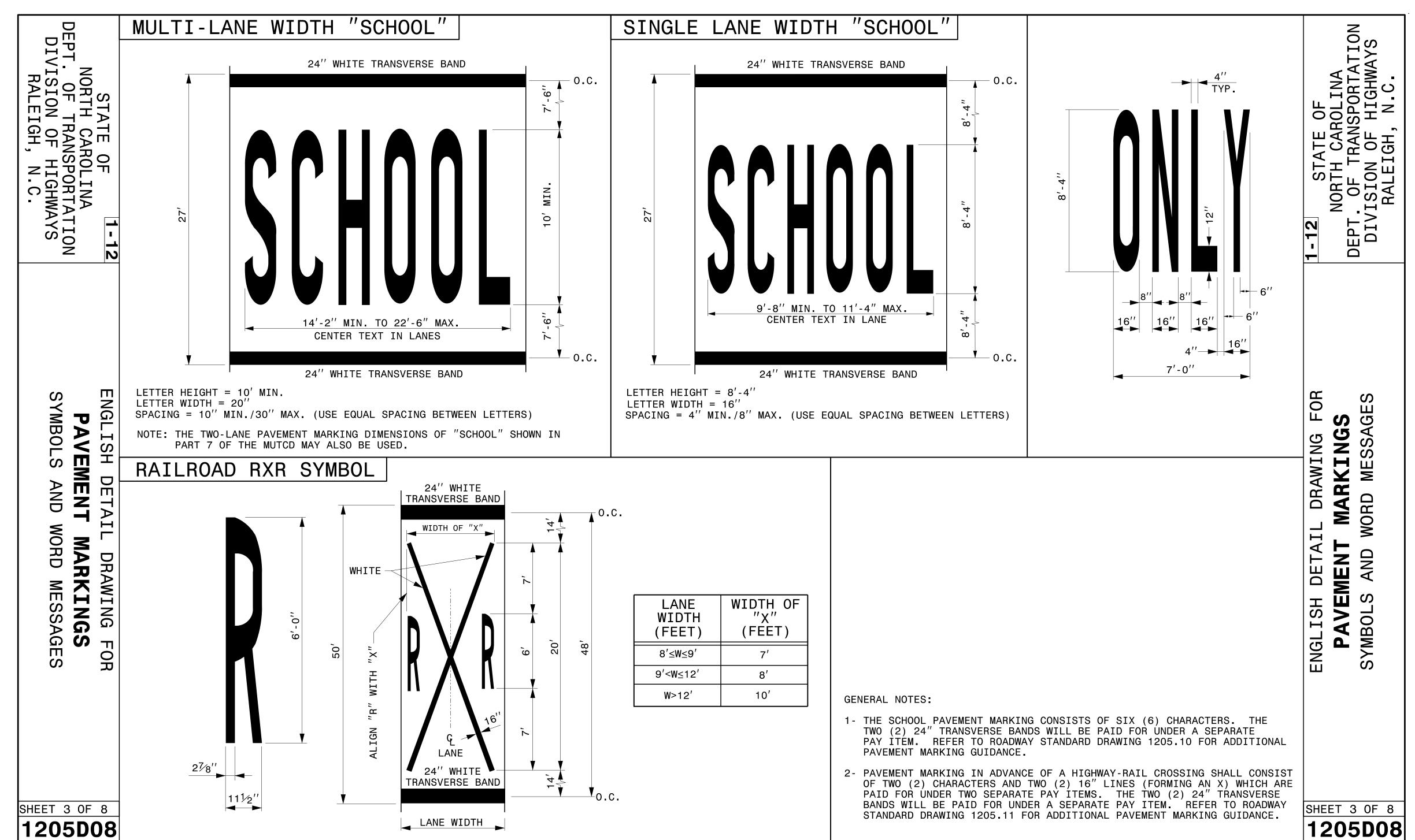
REVISED PAVEMENT MARKING ROADWAY STANDARD DRAWING
