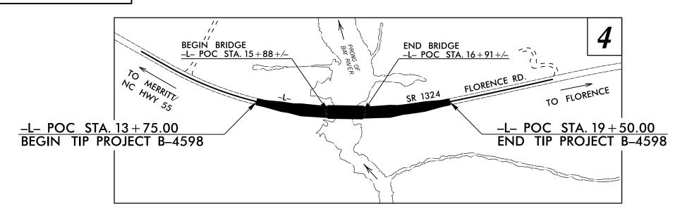
**DESIGN EXCEPTIONS** Horizontal SSD, Sta. 13 + 75 to Sta. 19 + 50 Superelevation, Sta. 13+75 to Sta. 19+50
