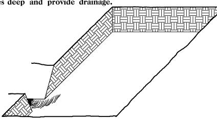
3. Backfill the trench with 2 inches well rotted sawdust. Place a 2 inch layer of well rotted sawdust at a sloping angle at one end of the trench.
