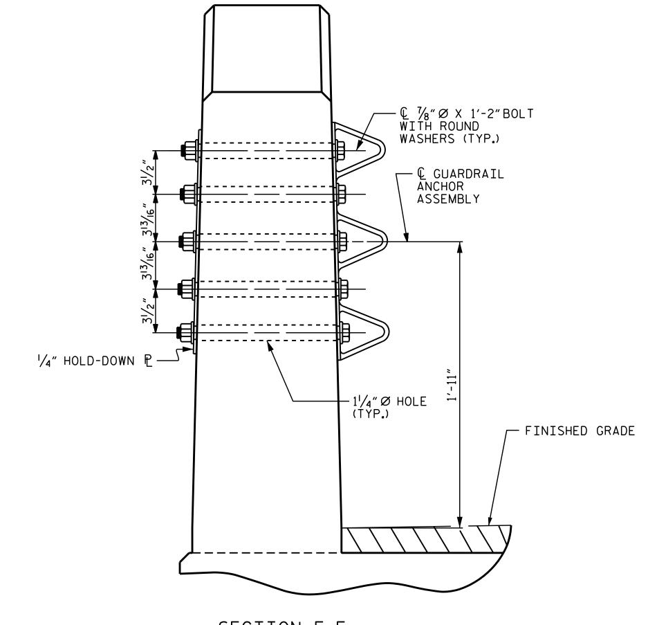
SECTION E-E GUARDRAIL ANCHOR ASSEMBLY DETAILS
