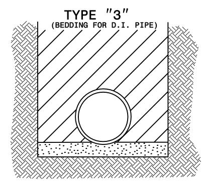
PIPE BEDDED IN 4" MINIMUM LOOSE SOIL. TRENCH BACKFILLED IN LOOSE 6" LAYERS COMPACTED TO TOP OF TRENCH USING LOCAL EXCAVATED MATERIAL IF APPROVED BY THE ENGINEER, OR SELECT MATERIAL ALL MATERIAL SHALL BE FREE OF ROCKS, FOREIGN MATERIAL, AND FROZEN EARTH. COMPACTION SHALL BE TO APPROX. 95% DENSITY IN ACCORDANCE WITH AASHTO T-99 AS MODIFIED BY THE DEPARTMENT OF TRANSPORTATION.
