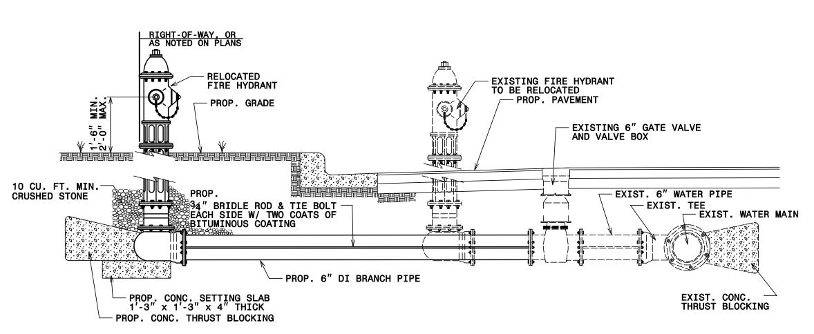
FIRE HYDRANT RELOCATION DETAIL
