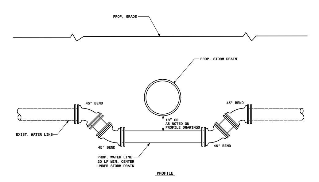
WATER MAIN RELOCATION (DOWN/UNDER) AT PROPOSED STORM DRAIN CROSSING
