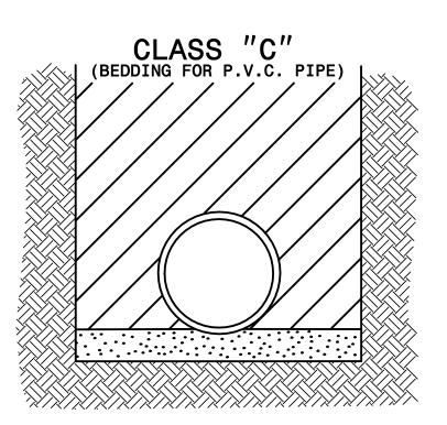
PIPE BEDDED IN LOOSE MATERIAL, LIGHTLY TAMPED WITH A MINIMUM OF 6" UNDER PIPE. TRENCH BACKFILLED IN LOOSE 6" LAYERS COMPACTED TO TOP OF TRENCH USING LOCAL EXCAVATED MATERIAL, IF APPROVED BY THE ENGINEER, OR SELECT MATERIAL. ALL MATERIAL SHALL BE FREE OF ROCKS, FOREIGN MATERIAL, AND FROZEN EARTH. COMPACTION SHALL BE TO APPROX. 95% DENSITY IN ACCORDANCE WITH AASHTO T-99 AS MODIFIED BY THE DEPARTMENT OF TRANSPORTATION.
