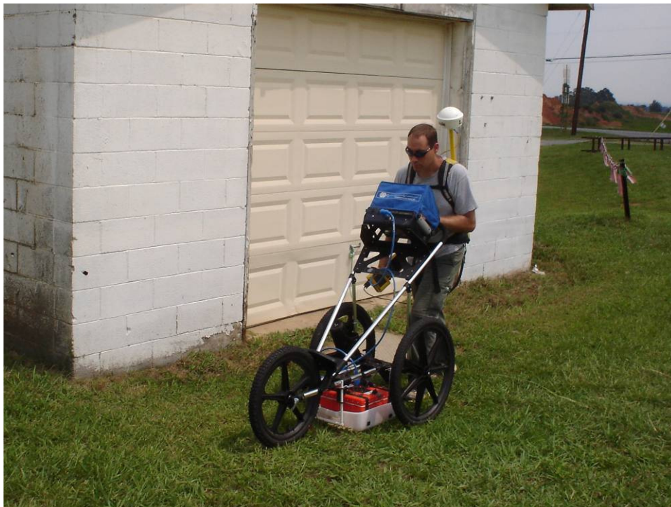
GSSI SIR-3000 Ground-Penetrating Radar with 400 MHz Antenna
