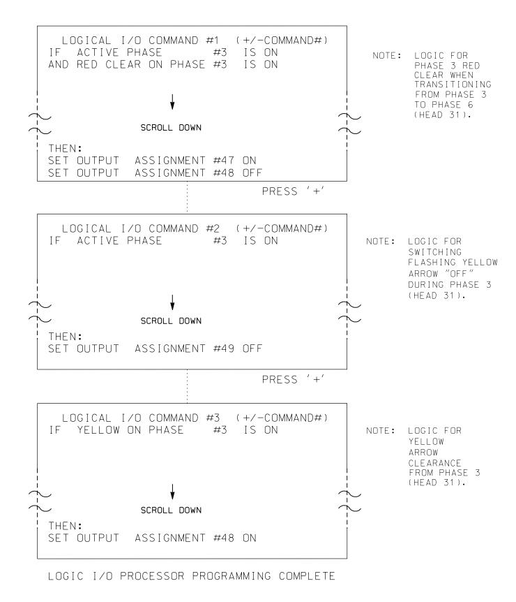
OUTPUT REFERENCE SCHEDULE USE TO INTERPRET LOGIC PROCESSOR OUTPUT 47 = Overlap B Red OUTPUT 48 = Overlap B Yellow OUTPUT 49 = Overlap B Green
