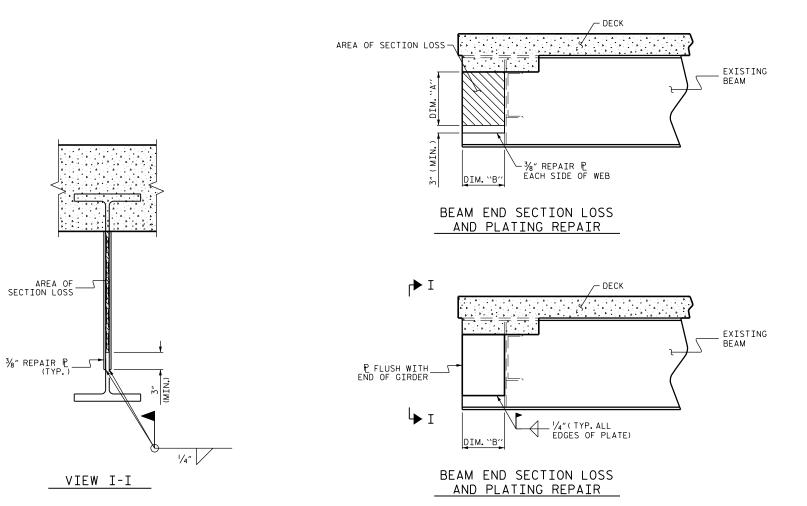
BEAM END PLATING REPAIR
