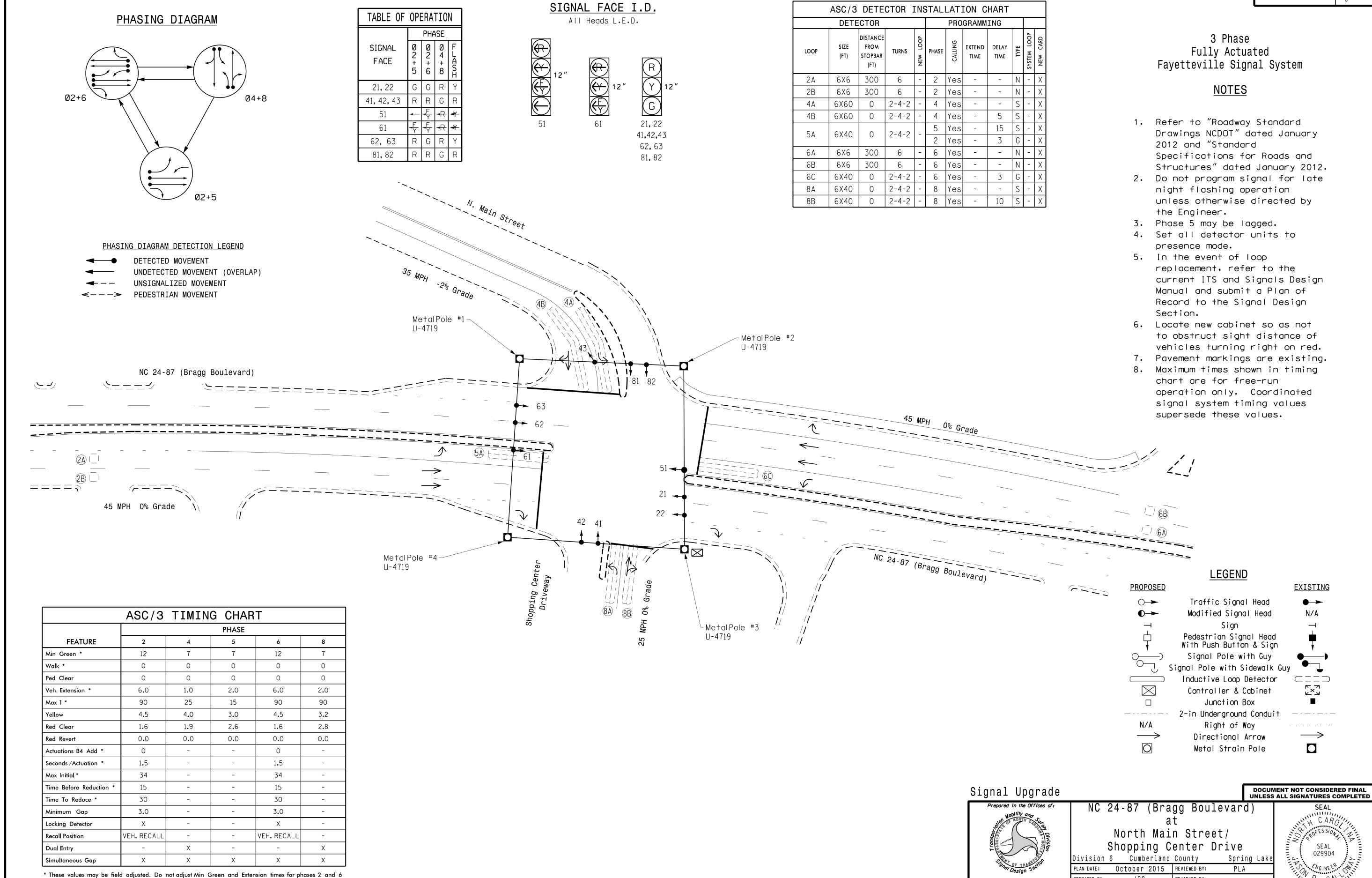
lower than what is shown. Min Green for all other phases should not be lower than 4 seconds.
