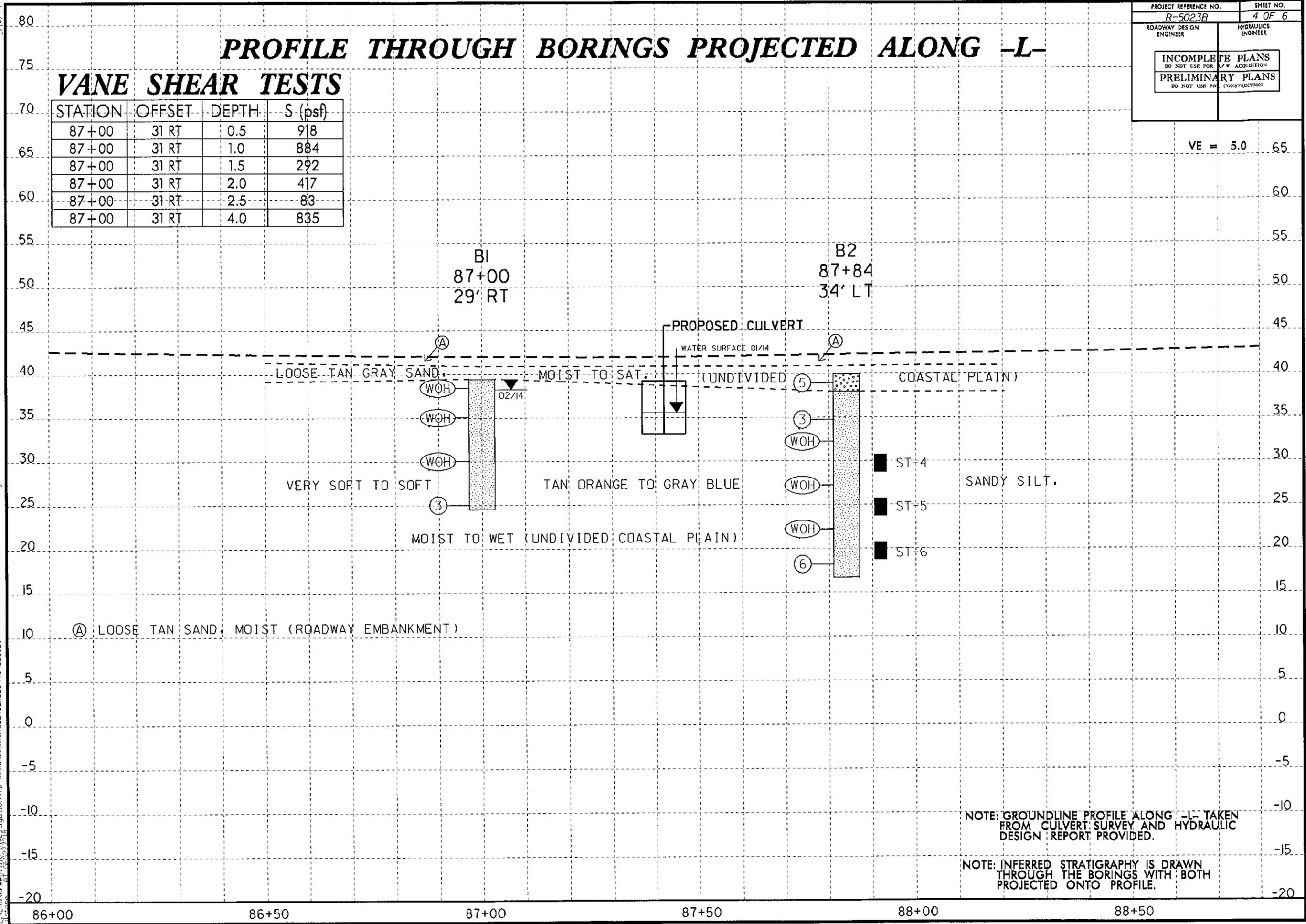
NOTE: GROUNDLINE PROFILE ALONG -L- TAKEN FROM CULVERT SURVEY AND HYDRAULIC DESIGN REPORT PROVIDED.
