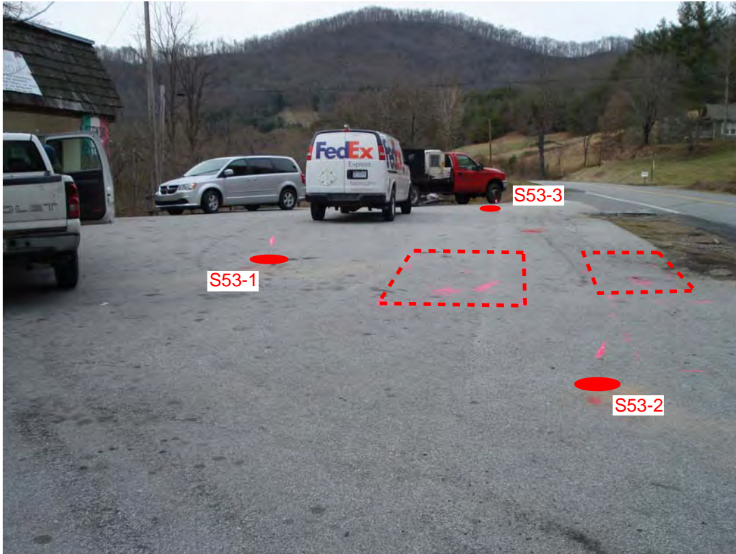
Photograph 3 : View looking south at locations of soil borings S53-1, S53-2, and S53-3, and locations of two identified GPR anomalies (dashed rectangles).
