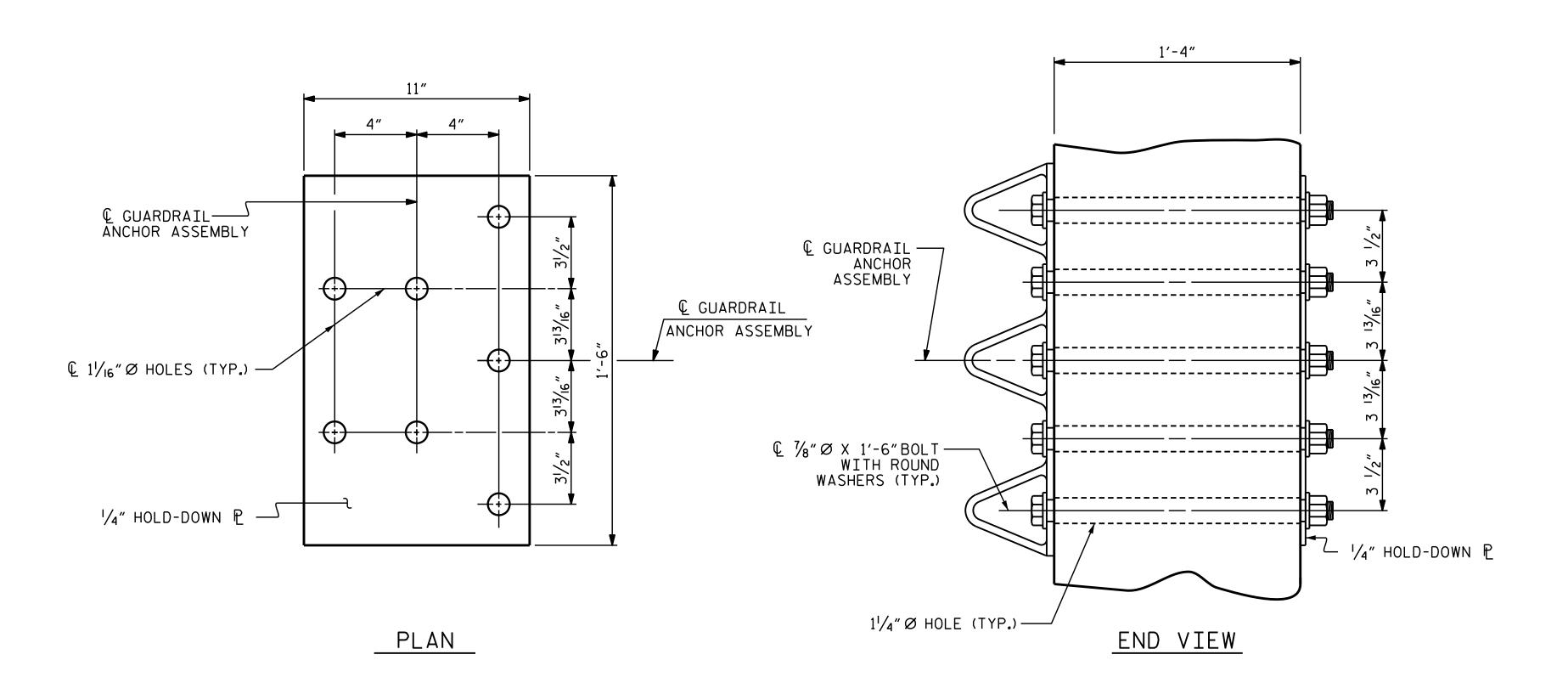
GUARDRAIL ANCHOR ASSEMBLY DETAILS
