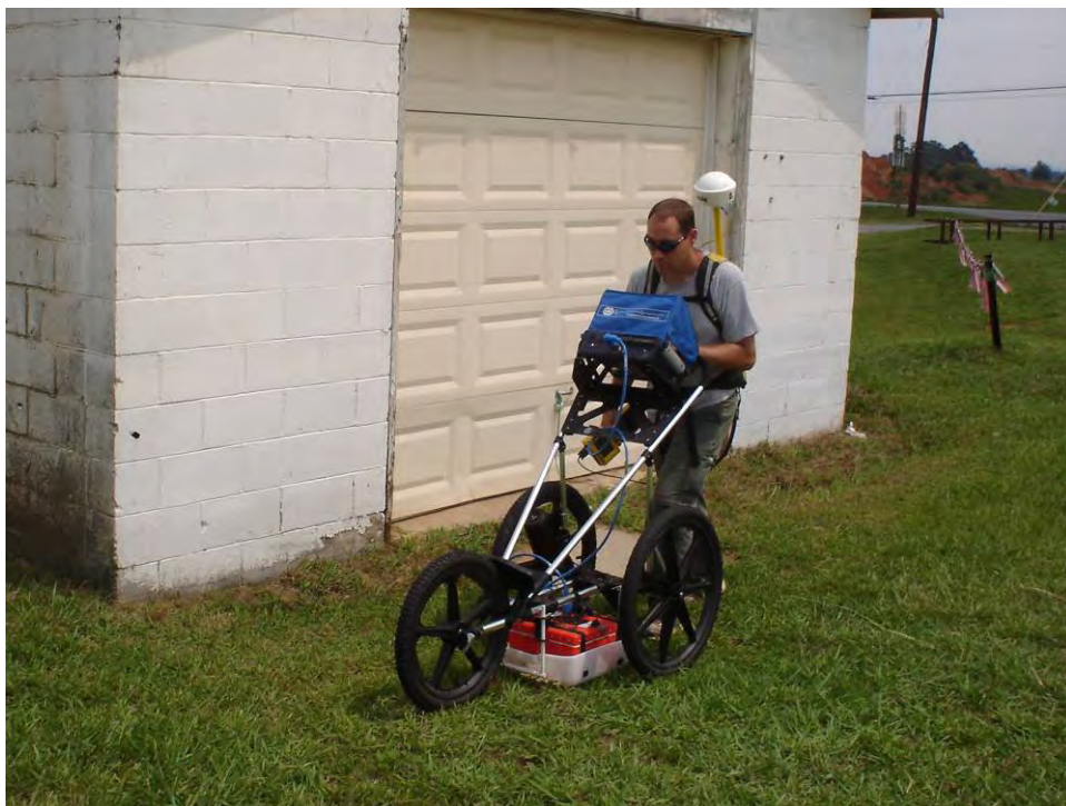
GSSI SIR-3000 Ground-Penetrating Radar with 400 MHz Antenna
