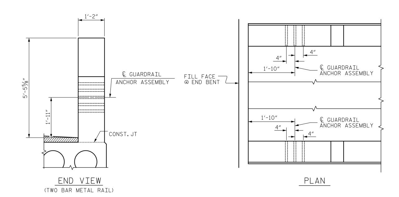
LOCATION OF GUARDRAIL ANCHOR AT END POST
