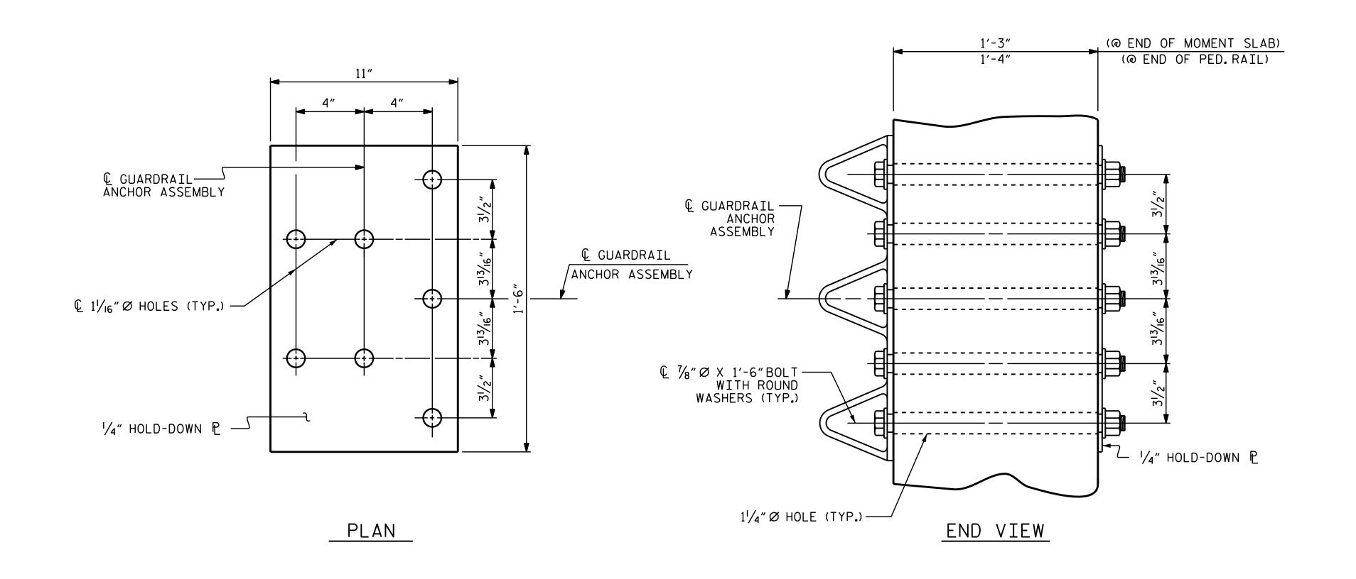
GUARDRAIL ANCHOR ASSEMBLY DETAILS
