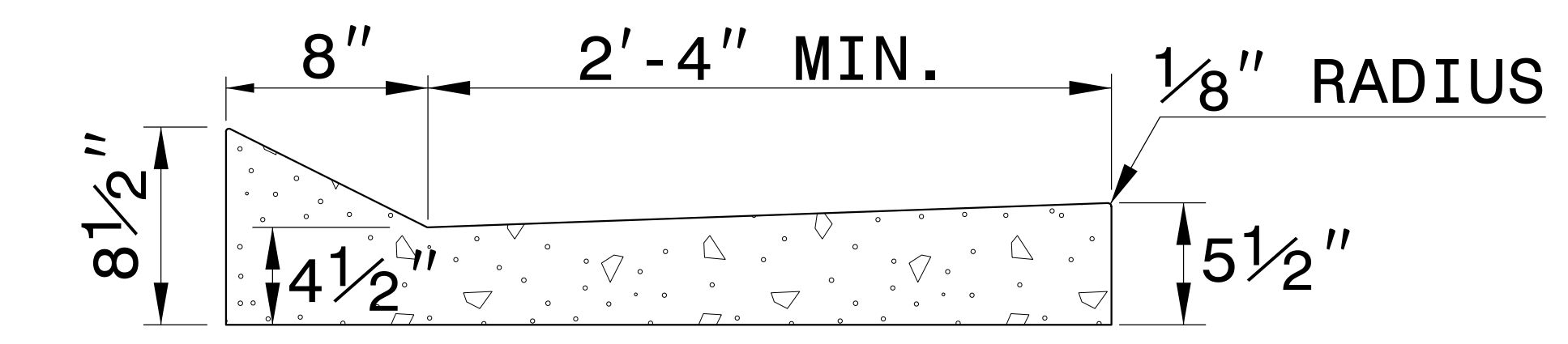
MODIFIED SHOULDER BERM GUTTER
