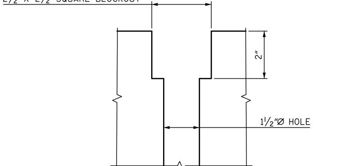
TYPICAL ANCHOR BLOCKOUT DETAIL
