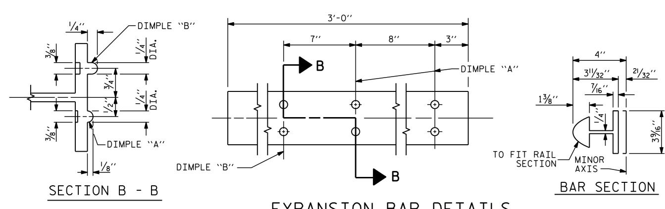
1/2" Ø [13 THREAD] HOLE FOR 1/2" Ø X 1" STAINLESS STEEL HEX HEAD CAP SCREW & 1/16" O.D., 17/32" I.D., 1/16" THICK WASHER (TYP.)
