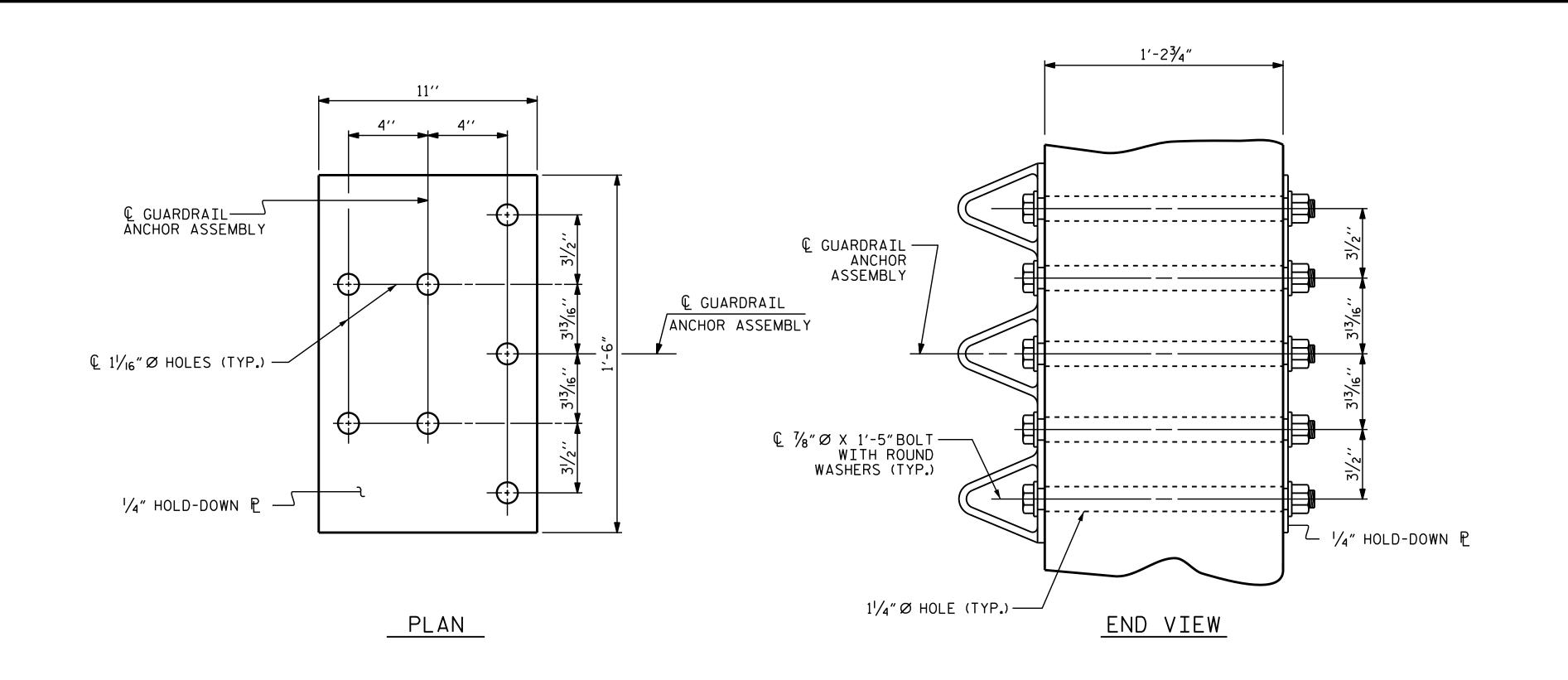
GUARDRAIL ANCHOR ASSEMBLY DETAILS
