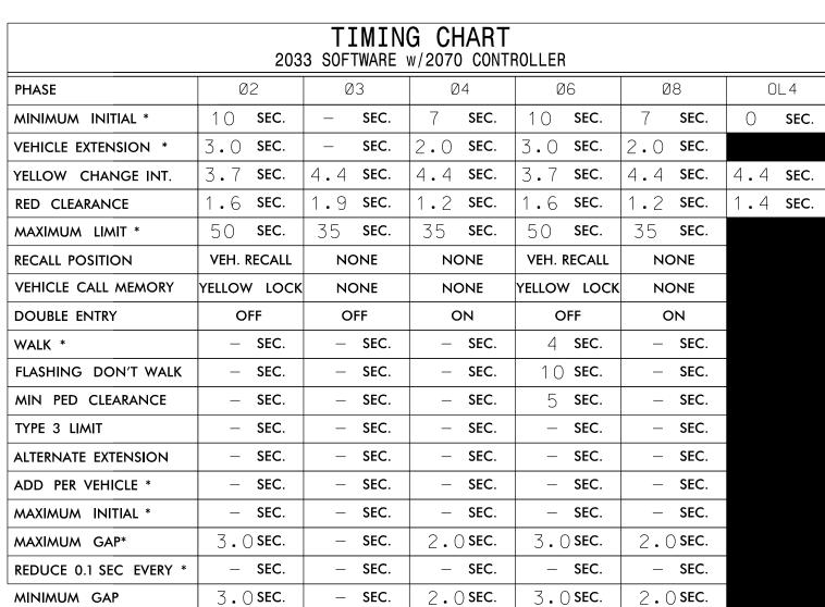
shown. Min Green for all other phases should not be lower than 4 seconds
