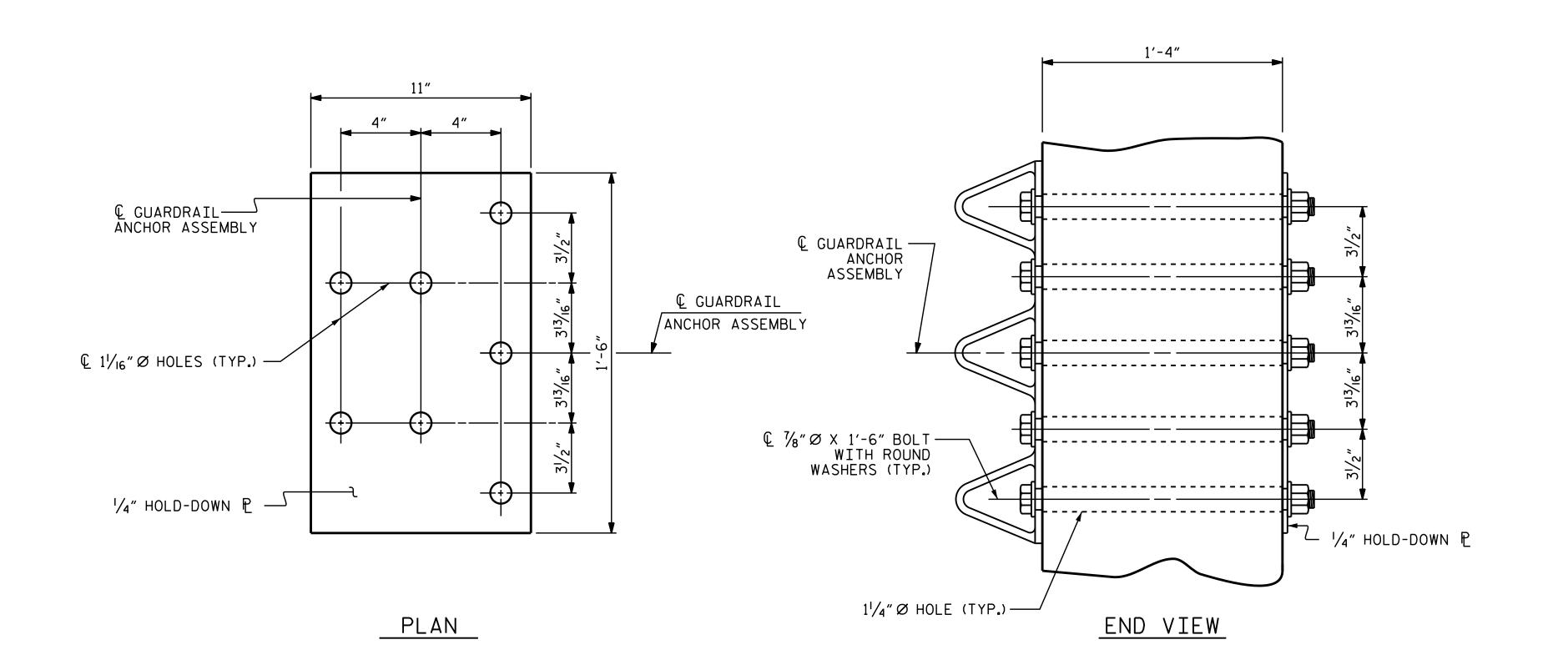
GUARDRAIL ANCHOR ASSEMBLY DETAILS
