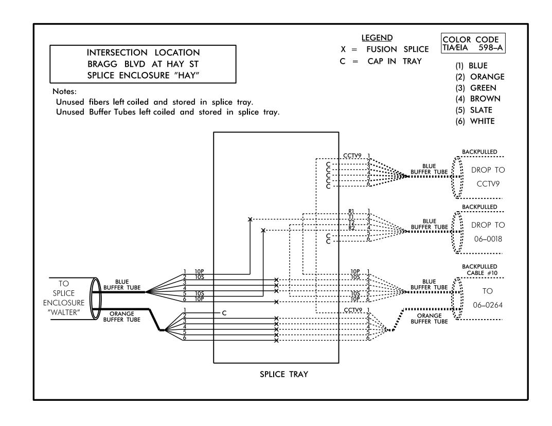
CONTRACTOR TO RECORD EXISTING SPLICE ARRANGEMENT FOR COMPARISON TO THE SUPPLIED SPLICE PLANS. IF DISCREPANCIES EXIST, CONTACT THE ENGINEER TO DETERMINE HOW TO PROCEED WITH RESPLICING.
